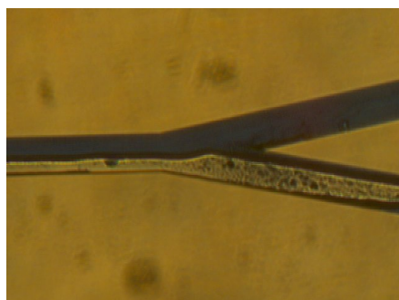
(c) Leakage of water to the toluene outlet. The Ca number of toluene is 2.18 \times 10^{-3} . The volumetric flow rate ratio ( \Phi_{aq}/\Phi_{org} ) of these two phases is 0.67.
