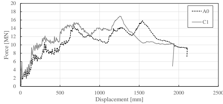
Figure 6.11: Reaction forces for elastoplastic-hardening material (C1) w.r.t. reference model (A0)
