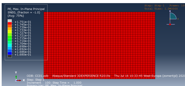
Figure E.2: PE principal strain at last increment where deformation is 80 mm.
