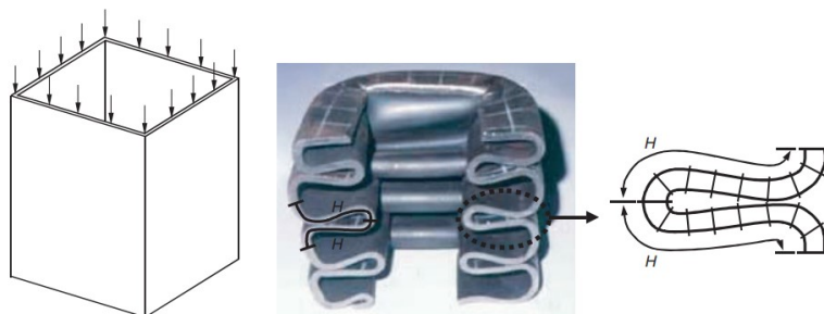
Figure 4.7: A thin-walled structure crushed under predominantly axial compressive loads and cut at its mid-section [51]
