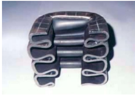
Figure 2.15: A plated structure crushed under axial compressive loads and cut at its midsection [53]
