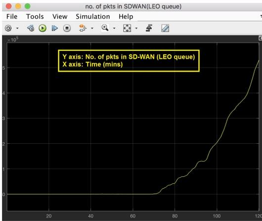
Figure 5.10: No. of pkts. in SDWAN (LEO Queue)- Simulation 1
