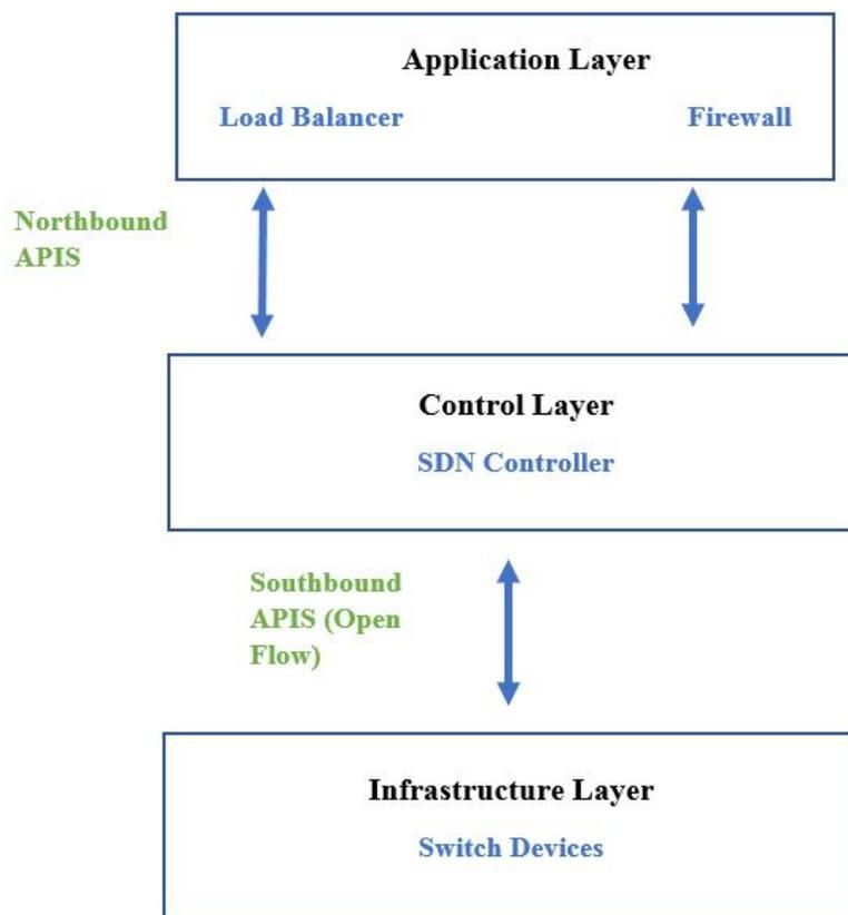
Figure 2.2: SDN Architecture Basic [9]
