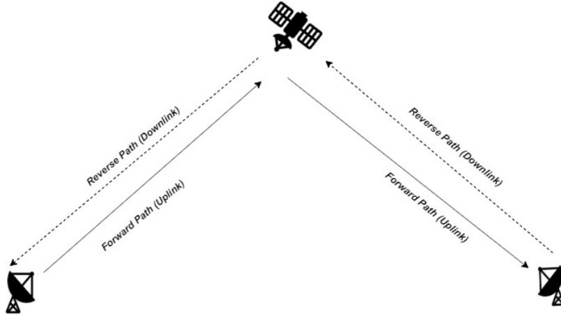
Figure 4.2: Uplink and Downlink in satellite network
