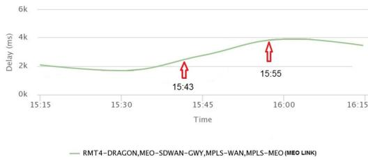
Figure 4.8: Delay (Forward Path Congestion)
