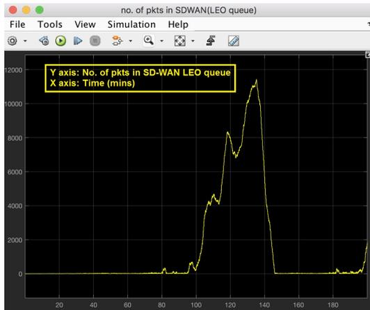
Figure 5.22: No. of pkts. in SDWAN (LEO Queue)- Simulation 2
