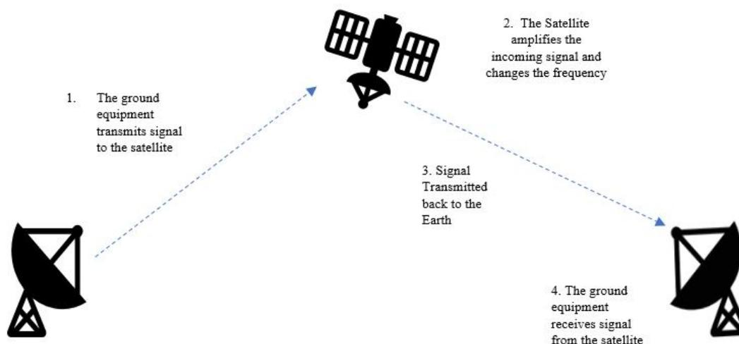
*Figure 1.1: Satellite Communication in 4 Steps [11]*
