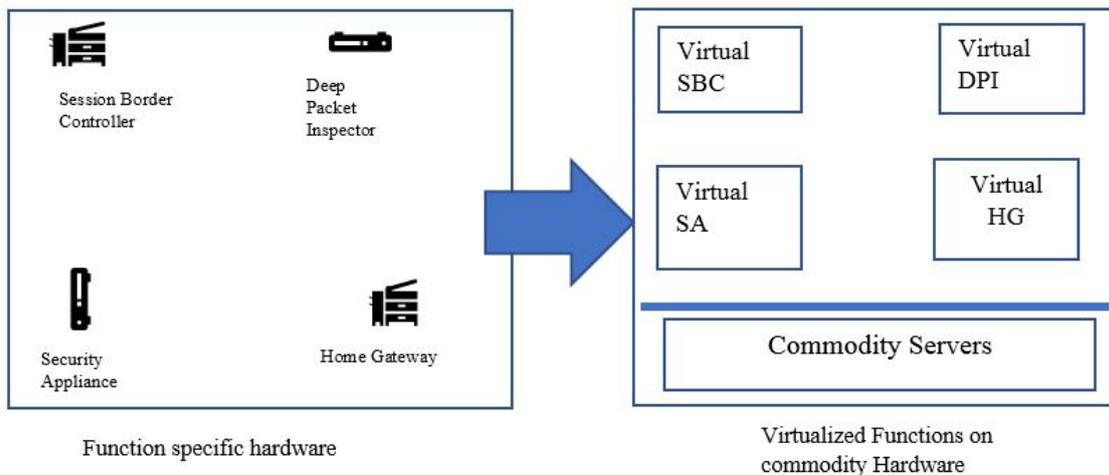
Figure 2.3: Network Function Virtualization concept [47]
