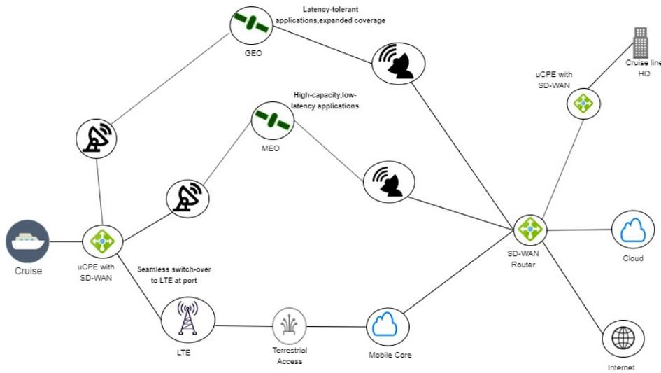
Figure 5.1: SD-WAN based multi-access network on a cruise ship [5]
