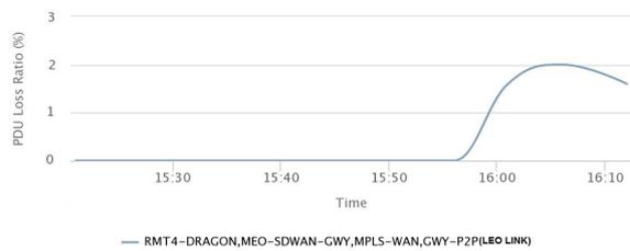
Figure 4.21: PDU loss at LEO link
