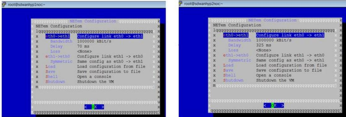
Figure 4.5: Changing Parameters in Hypervisor 1(MEO), Hypervisor 2 (GEO)
