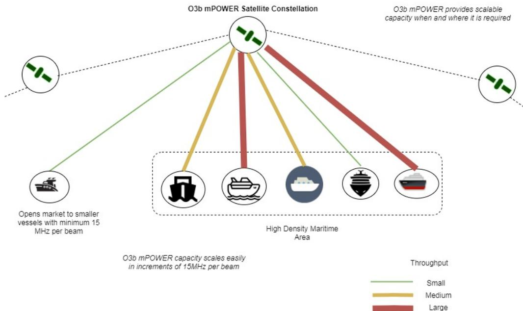
Figure 3.2: O3b mPOWER capacity scaling capabilities
