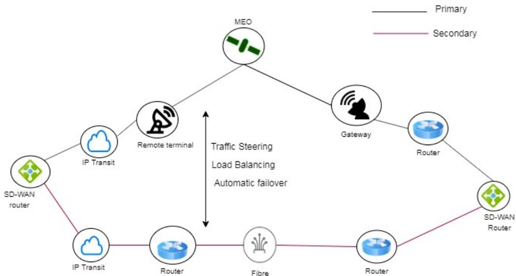
Figure 2.8: SDWAN based hybrid MEO-terrestrial network [5]
