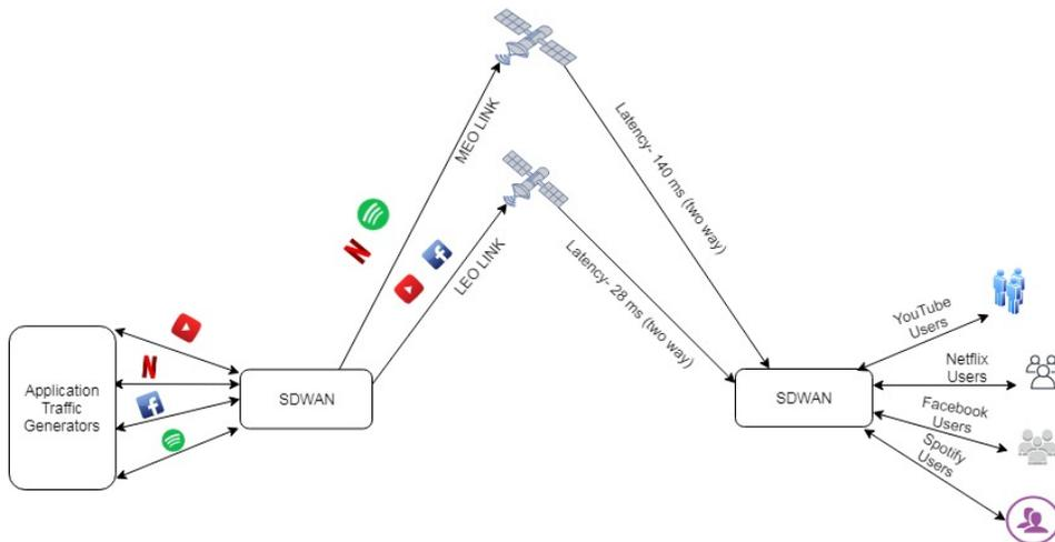
Figure 5.2: Simulation Setup Representation
