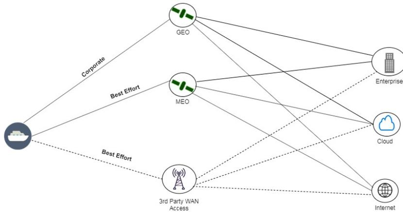
Figure 1.2: Current method of Managing WAN connections
