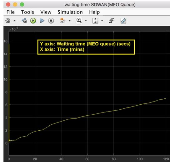
Figure 5.17: Waiting time SDWAN (MEO Queue) ( $\Delta t_1$ )- Simulation 1
