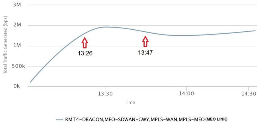
Figure 4.13: Total Traffic Generated Rate (Bidirectional Congestion)
