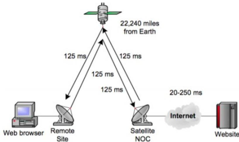
Figure 4.1: Total Round-Trip Time using Broadband Satellite [48]
