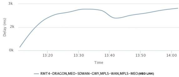
Figure 4.16: Delay at MEO link (Without Algo)
