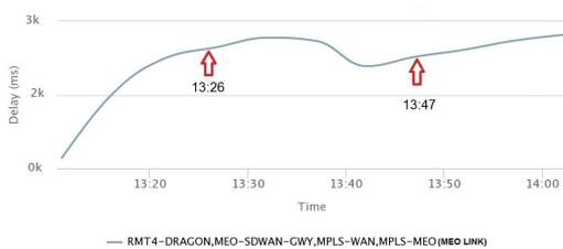
Figure 4.14: Delay (Bidirectional Congestion)
