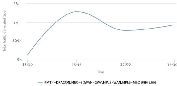
Figure 4.22: Total Traffic Generated Rate MEO link (With Algo)
