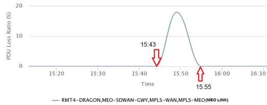
Figure 4.9: PDU loss Ratio (Forward Path Congestion)
