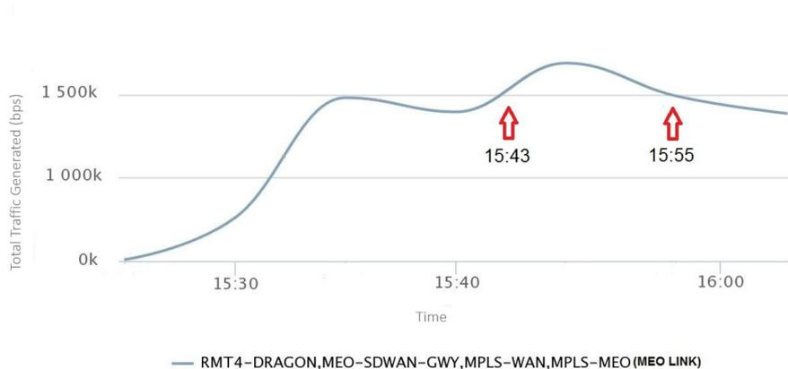
Figure 4.7: Total Traffic Generated Rate (Forward Path Congestion)
