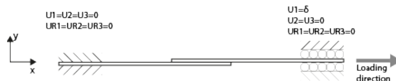
Figure 4. Boundary conditions for the FE analyses.
