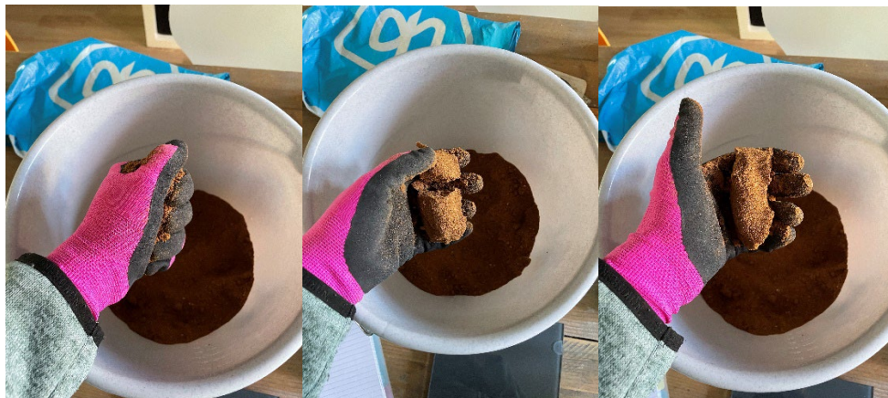
Figure 4. Wetted loam, left squeezing. Middle forms a ball, but breaks so needs more water. Right holds shape and feels sticky, good to use for next step.
