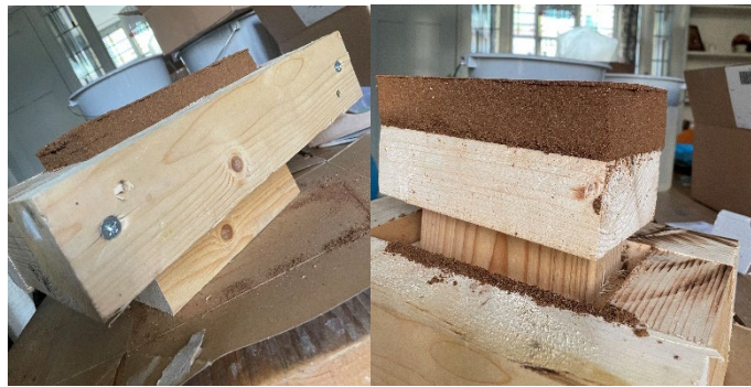
Figure 6. Left, turn mold upside down and place a smaller block under the pressingblock. Right, slowly press the mold down until the loambrick is free.
