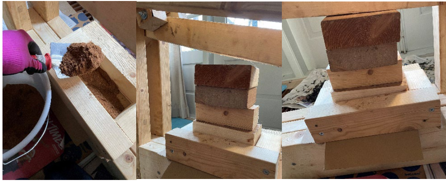
Figure 5. Left, fill mold. Middle stack until underbeam of lever mechanism is reached. Right press down on lever.
