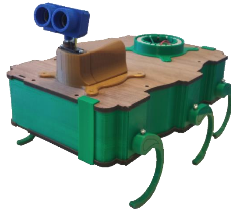
Figure 20: Zebro fitted with ultrasonic module
