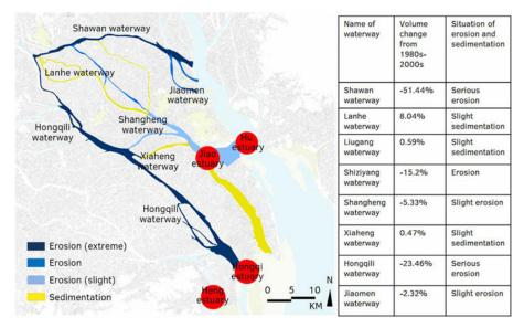
FIG. 4.37 The status of Erosion and sedimentation of waterways in Nansha area
