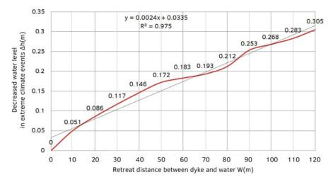
FIG. 5.32 The relationship between the retreat distance from dyke to shoreline and decreased water level of waterways under extreme climate change condition.
