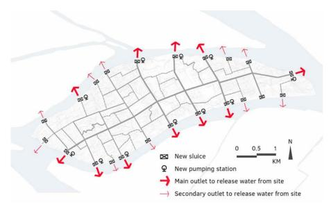
FIG. 5.40 Proposal for new sluices and pumping stations
