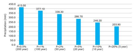
FIG. APP.D.2 The prediction of max daily precipitation under different climate scenarios . (Source: Author mapped based on Contour Map of Heavy Precipitation Parameters for Planning and Design, 2018)
