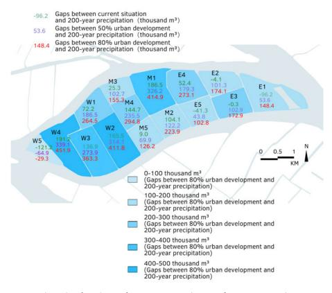
FIG. 5.20 The number of gaps between future precipitation and capacity of water storage in each water collective unit
