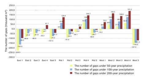
FIG. 5.42 The number of gaps between the capacity of water storage and future precipitation under current situation (unit: thousand m<sup>3</sup>)
