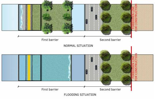
2 The situation of buffering belt under normal and flooding situation
