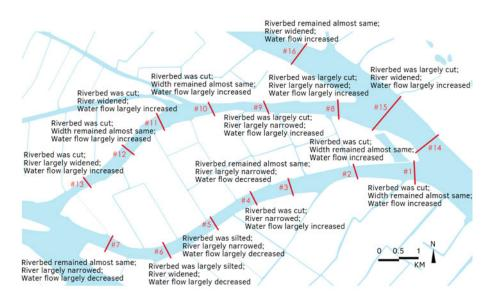
FIG. 5.12 The condition of sedimentation (erosion) of waterways
