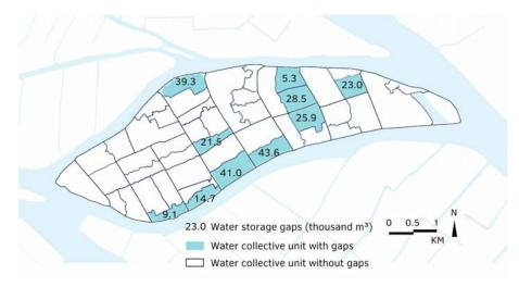
FIG. 5.46 The number of gaps between the capacity of water storage and future precipitation without the consideration of pre-descent water level (presented in space, unit: thousand  $m^3$ ).
