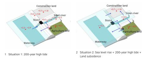
FIG. 5.16 Relationship between the changing water level of waterways, inner-rivers and dyke's height under two situations
