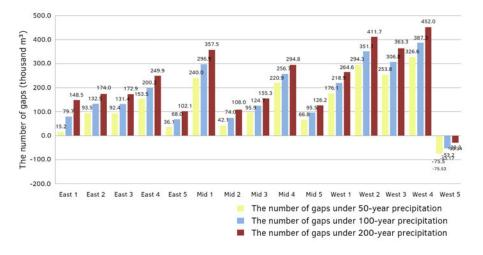
FIG. 5.44 The number of gaps between the capacity of water storage and future precipitation under 80% urban development (unit: thousand m<sup>3</sup>)
