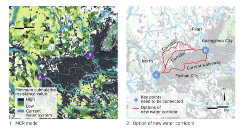
FIG. 4.28 Options of new water corridors based on MCR model
