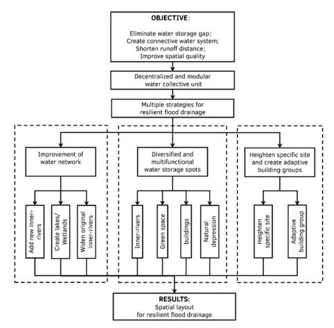
FIG. 5.24 Technical route for resilient flood drainage
