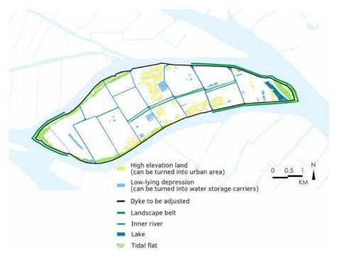
FIG. 5.21 Potential elements to be organized for flood control and drainage
