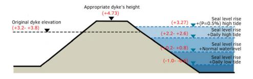
FIG. 5.30 Appropriate height of dyke
