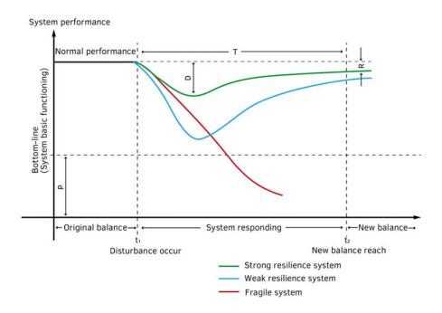
FIG. 2.4 The schematic diagram of resilient process
