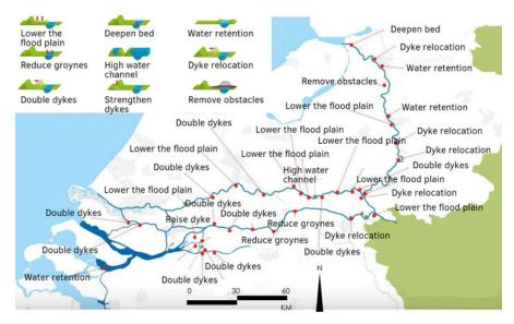
FIG. APP.B.4 Diversified sections applied in the project of 'Room for Rivers'. (Source: Ruimtevoorderivier, 2014)
