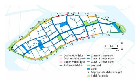
FIG. 5.36 Spatial layout for flood control and drainage
