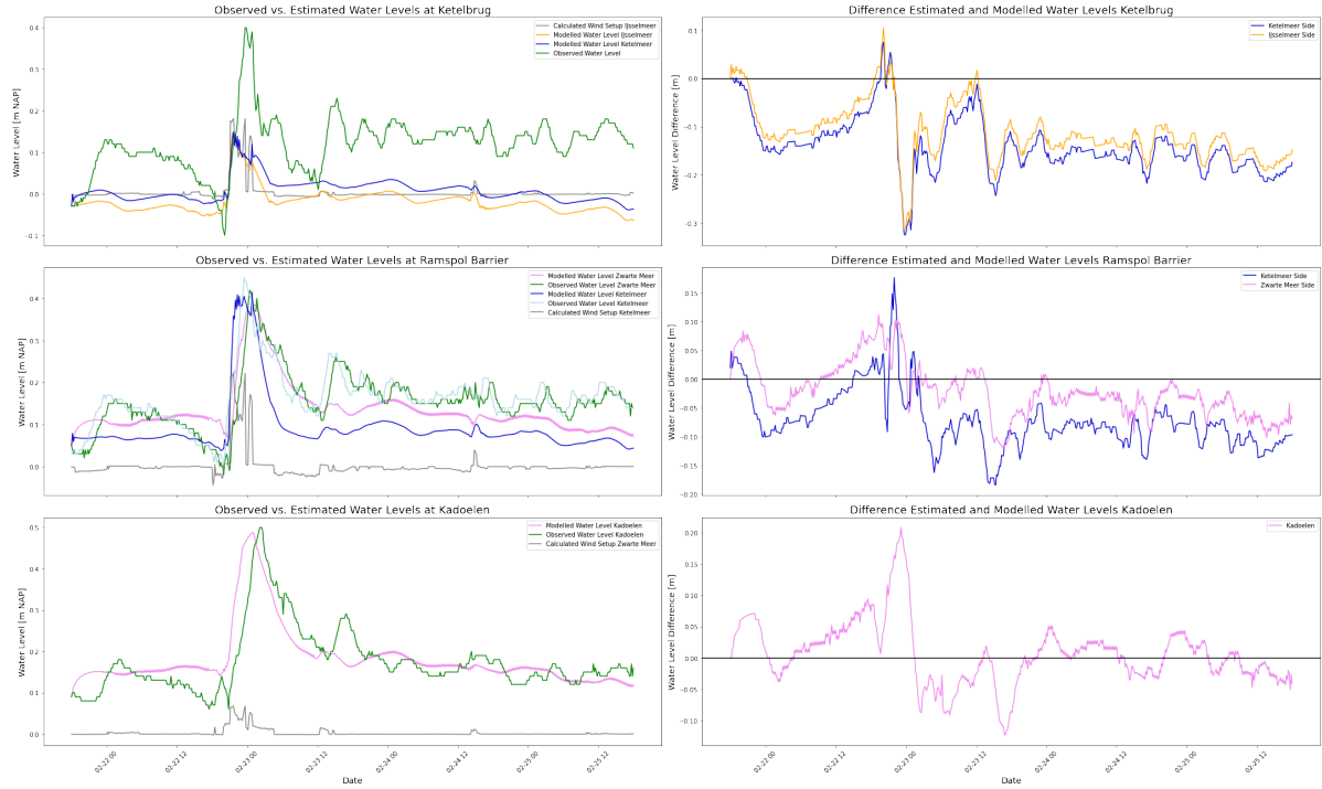
Figure C.18: Calibration results of the peak of February 23, 2024 with \tau_{ij} = 322.47 , \tau_{km} = 6511.14 , and \tau_{zm} = 296.53 .
