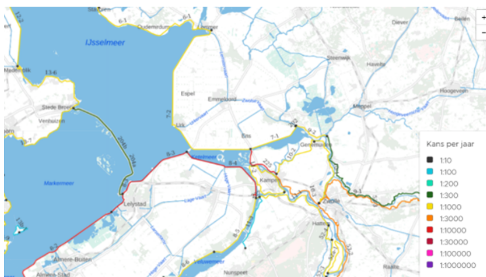
Figure 2.9: Lower Limit Standard of Primary Flood Defences in the Water System (van Infrastructuur en Waterstaat, n.d.).
