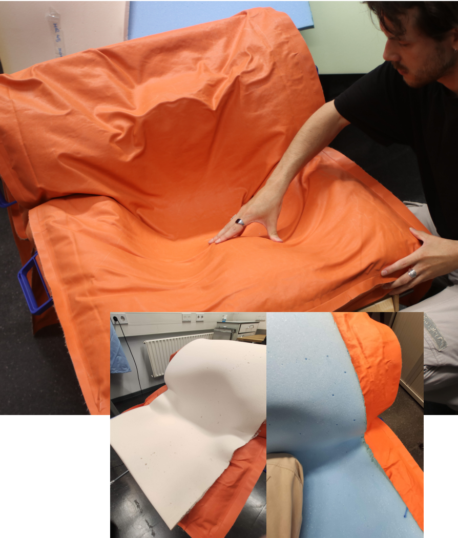
figure 16: 20 mm foam (left) and 30 mm foam (right) but adapt well to the shape of the body
