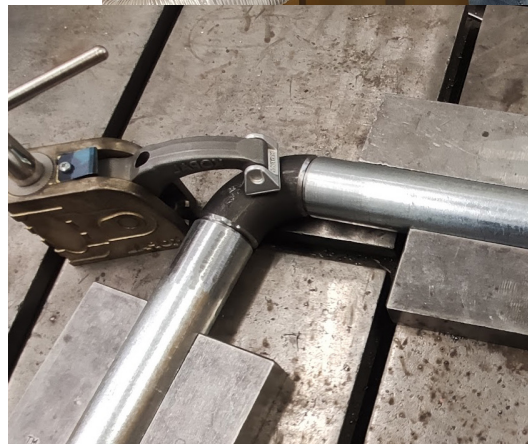
figure 74: smoothing the welds to imitate a bent frame
