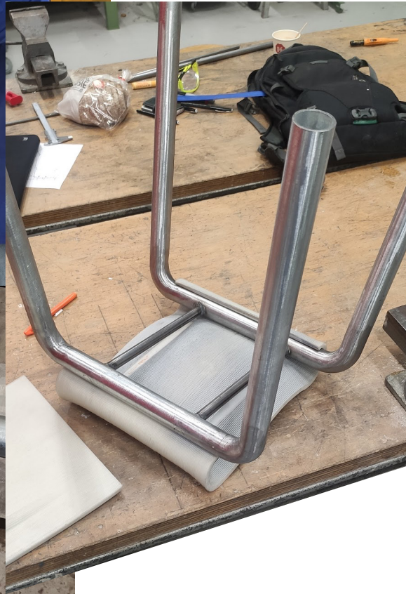
figure 75: the fit of the leg frame turned out to be too tight for the connection piece
