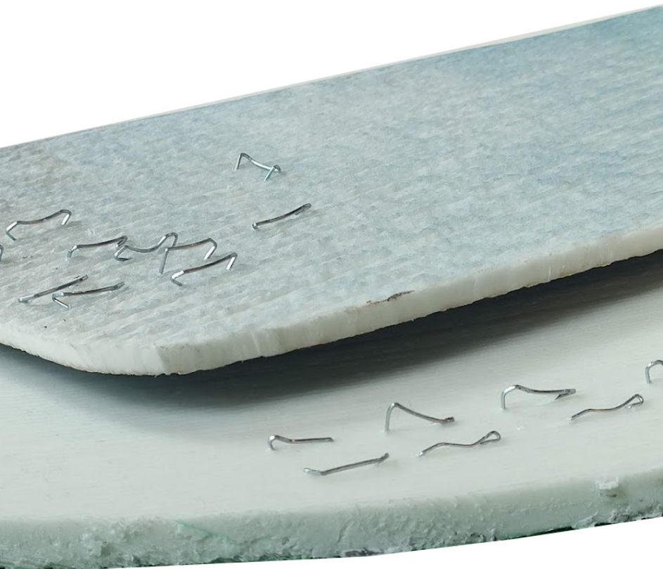
figure 24: staples not failing with electronic tackers
