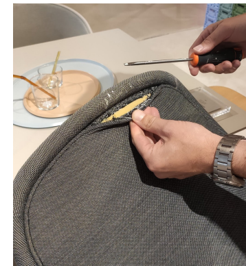
figure 22: blind seam profile figure 23: the working of the blind seam profile illustrated in practice
