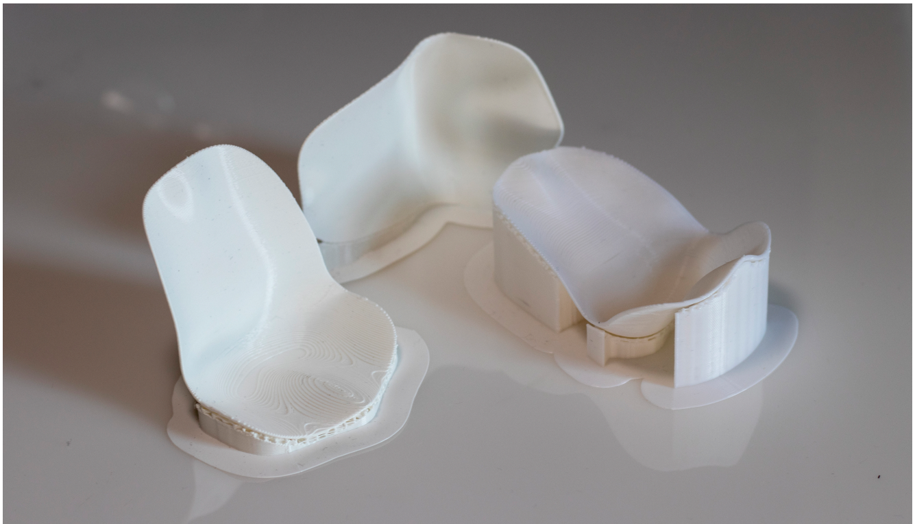
figure 27: printing scale models in differing orientations
