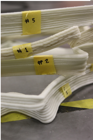
figure 70: various samples with varying layer heights.
