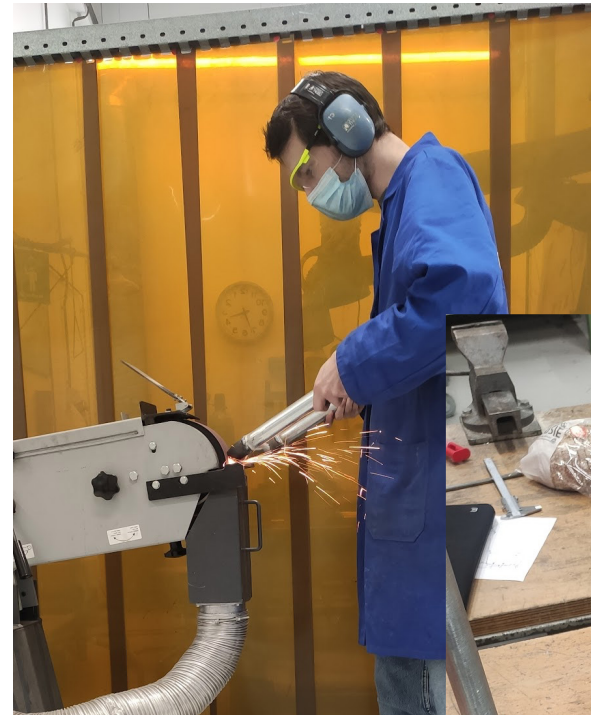
figure 74: smoothing the welds to imitate a bent frame
