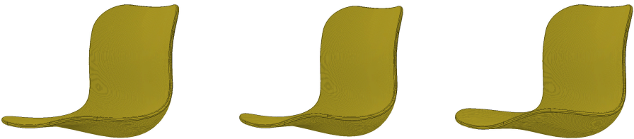
figure 45: from left to right, the seat shape increases in visual balance and flow, while becoming less accurate
