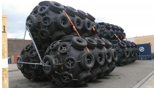
Figure 5.7: Triangular Yokohama connection [65]
