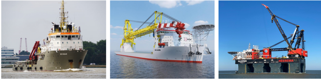
Figure 2.19: FOWT installation vessels: Tug (left), Heavy-Lift Vessel (middle), and Semi-Submersible Crane Vessel (right) [57] [46] [74]
