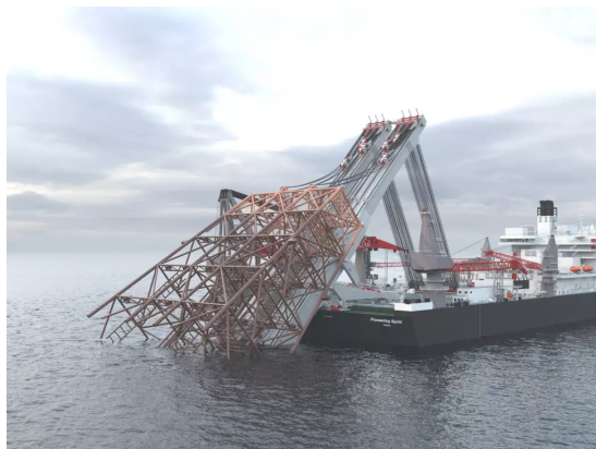
Figure 3.3: Jacket Lift System during operation [84]
