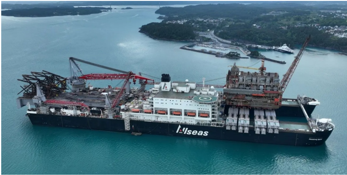
Figure 1.5: Pioneer Spirit transporting a decommissioned topside and jacket, courtesy of Allseas
