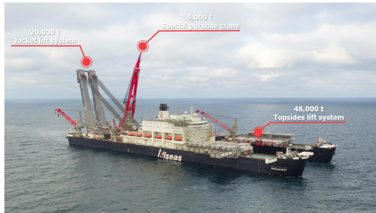
Figure 3.1: Topsides Lift System, Jacket Lift System, 5000t special purpose crane, courtesy of Allseas
