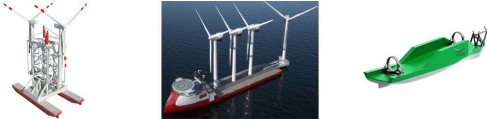
Figure 2.20: Conceptual FOWT installation vessels [47] [40] [51]
