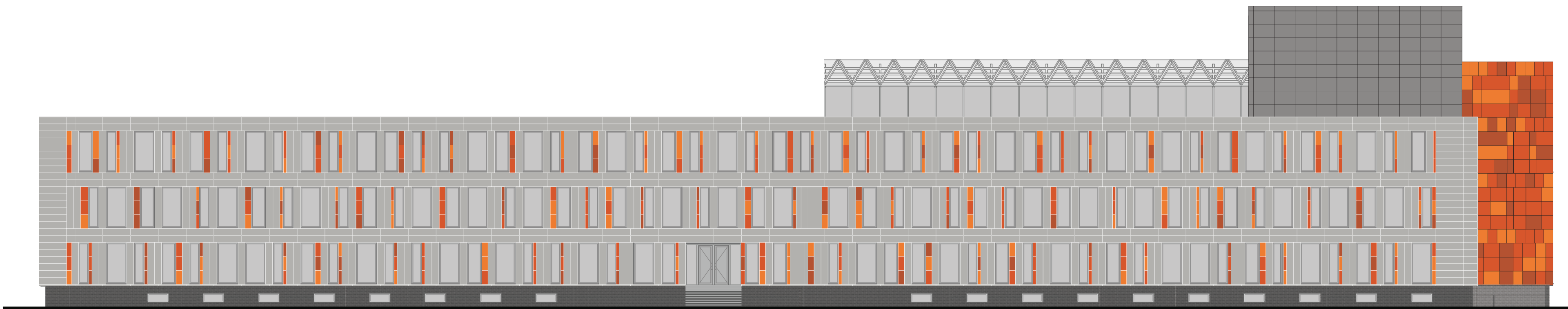
1:200 REUSED MATERIALS FACADE ALONG THE AULA
