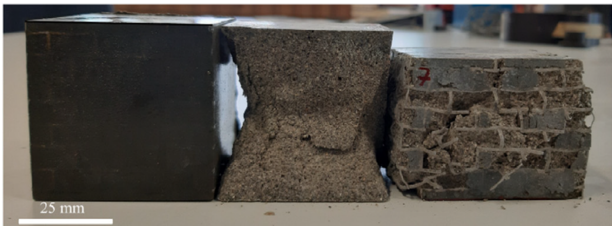
Figure 1.2: Composite behavior of an auxetic lattice as steel reinforcement for a concrete element [29]
