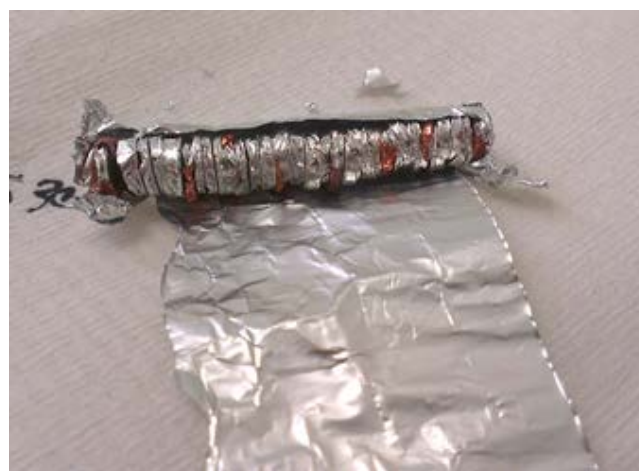
Figure 3. Packing sequence for irradiation. Difference between standards and unknowns is obvious from the copper around the standard samples. The total length of this wrap is 5 cm.
