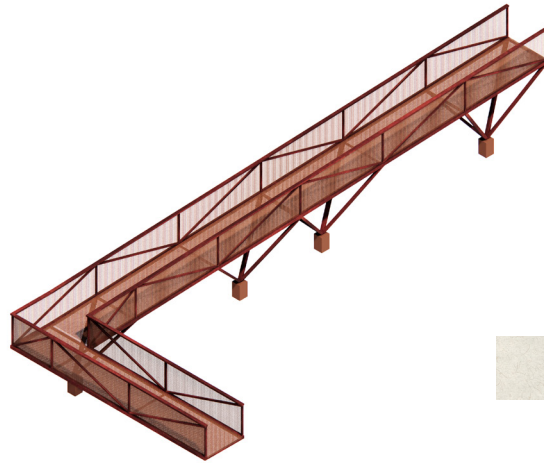
PLANAR STEEL FRAME WITH WITH TREE-LIKE FOOTING
