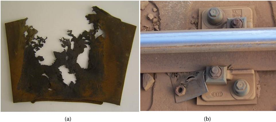
Figure 4.3: Worn railpads from Dutch railway. (a) Example one of worn railpad; (b) Example two of worn railpad.
