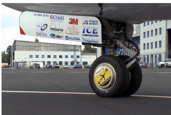
(a) Wheeltug system implemented in NLG, source: Wheeltug
