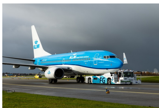
(b) KLM Boeing 737 being towed by TaxiBot, source: KLM
