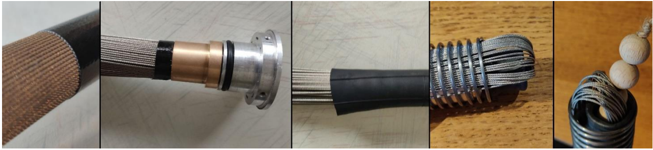
Figure 4.14: Assembly of the initial prototype in five steps from left to right until the point where the fibers were unable to evert around the tip of the inverted tube.
