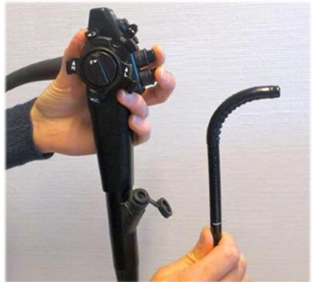
Figure 1.1: A state of the art flexible endoscope with a tip on the anterior end (right), a control handle on the posterior end (left) and a flexible tube or shaft, connecting the two. From: E.D. Rozeboom, et al. [3].
