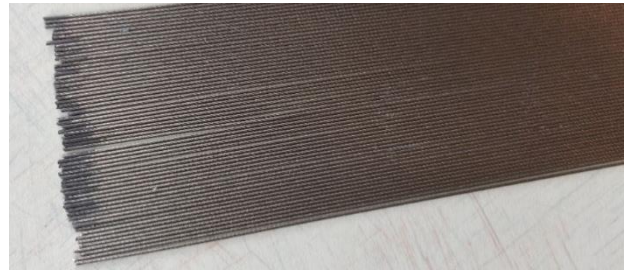
Figure 4.8: Steel fibers, cut to size and glued at the ends to prevent fraying of their 7x7 strand configuration.
