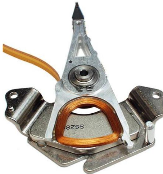
Figure 5.3 - A rotary voice coil from a Seagate harddisk. [33]
