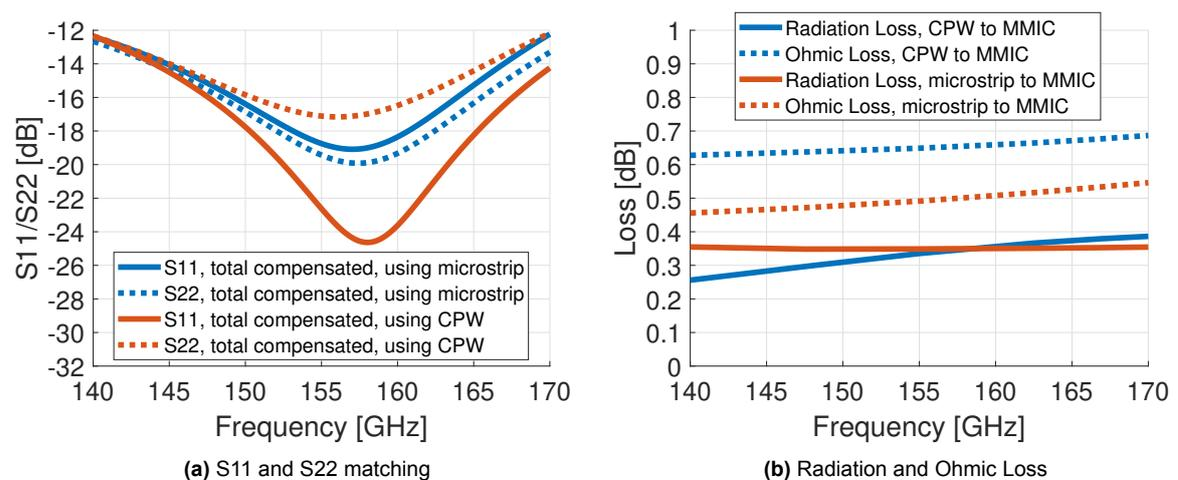
**Figure 4.10:** Simulated performance (from full-wave CST simulation) of the via-less flip-chip microstrip interconnection to the MMIC after adding a high impedance series transmission line (from Fig. 4.9b) in blue versus the CPW interconnection to the MMIC after adding compensation (from Fig. 4.5), plotted in red.
