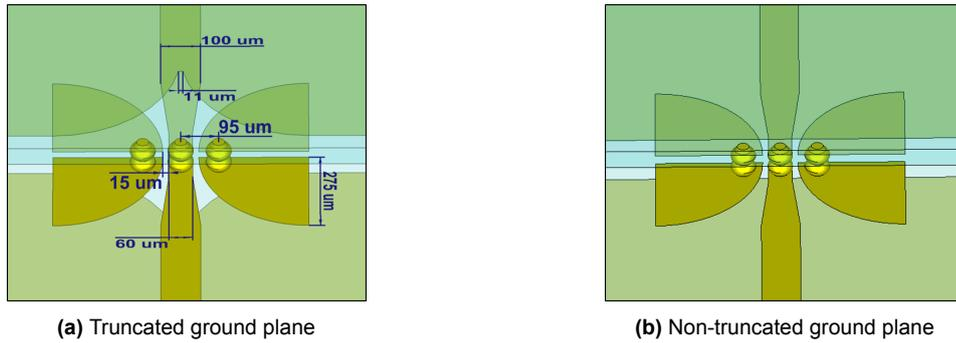
Figure 2.8: 3D model of the via-less Flip-Chip microstrip interconnection
