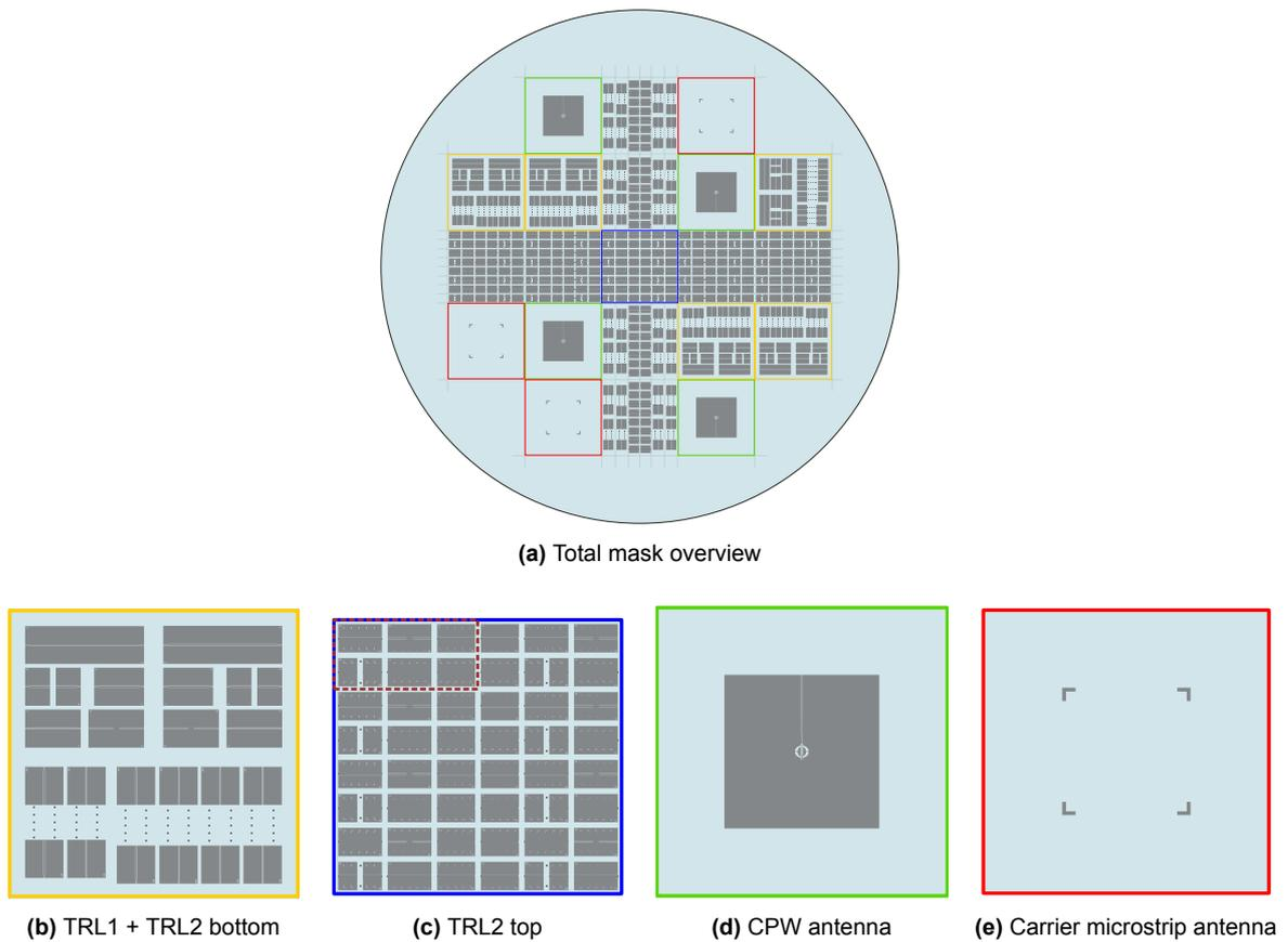
**Figure 3.12:** CPW mask design on 4 inch  $500\mu\text{m}$ -thick fused silica wafer using aluminum metallization.
