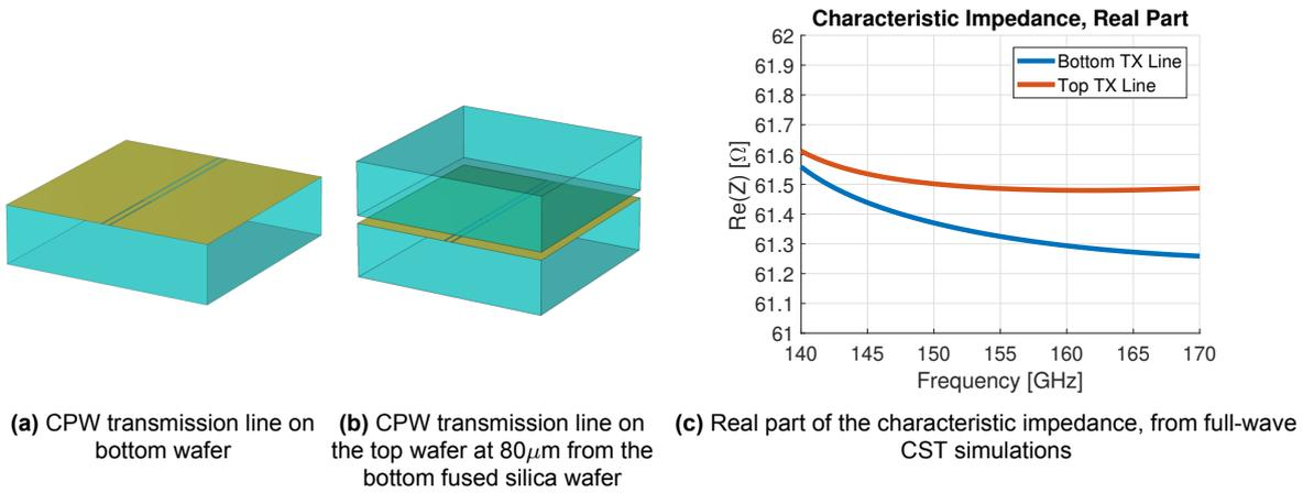
**Figure 2.3:** CPW transmission lines for the flip-chip interconnection.
