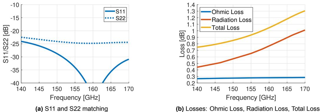
**Figure 2.7:** Simulated performance of Flip-Chip microstrip interconnection using vias.
