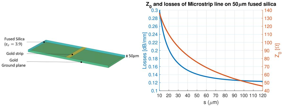
**Figure 1.10:** 3D view of a  $50\ \Omega$  microstrip transmission line on fused silica of thickness  $50\ \mu\text{m}$  **Figure 1.11:** Characteristic impedance and losses of a microstrip line on  $50\ \mu\text{m}$  fused silica wafer.
