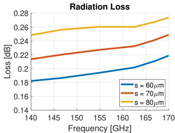
**Figure 2.2:** Radiation loss for varying CPW width for the flip-chip interconnection using CPW transmission lines
