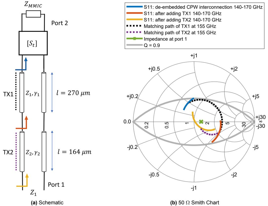
**Figure 4.4:** CPW interconnection to the MMICs including high impedance transmission line compensation.
