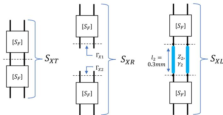
Figure 3.10: Schematic of TRL2 using S-parameter boxes
