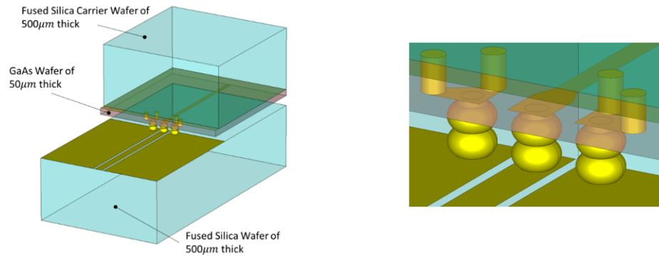
(a) 3D model of the flip-chip interconnection between the MMICs and transmission line in fused silica
