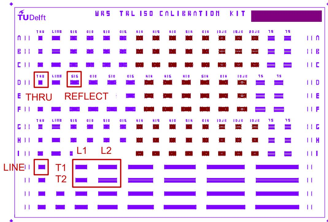
**Figure A.1:** Total mask used for preliminary TRL measurements. Blue indicates aluminum and red is a resistive layer, not relevant for the measurements. Red boxes indicate the measured features.
