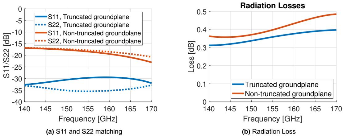
**Figure 2.10:** Simulated performance of via-less flip-chip microstrip interconnection for truncated and non-truncated ground plane.
