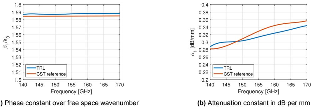
**Figure 3.4:** Propagation constant results: using TRL1 equations from simulated TRL1 structures (blue) and simulation of a uniform reference line (red).
