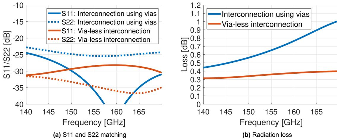
**Figure 2.15:** Comparison of S11/S22 matching and radiation loss between the flip-chip microstrip interconnection using vias and the via-less interconnection.
