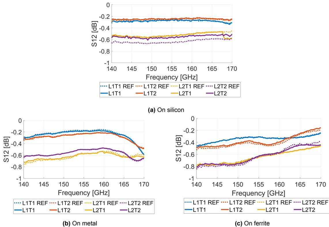
**Figure 5.3:** Verification of the TRL and Switch-term correction implementation in MATLAB against the WinCal TRL reference.
