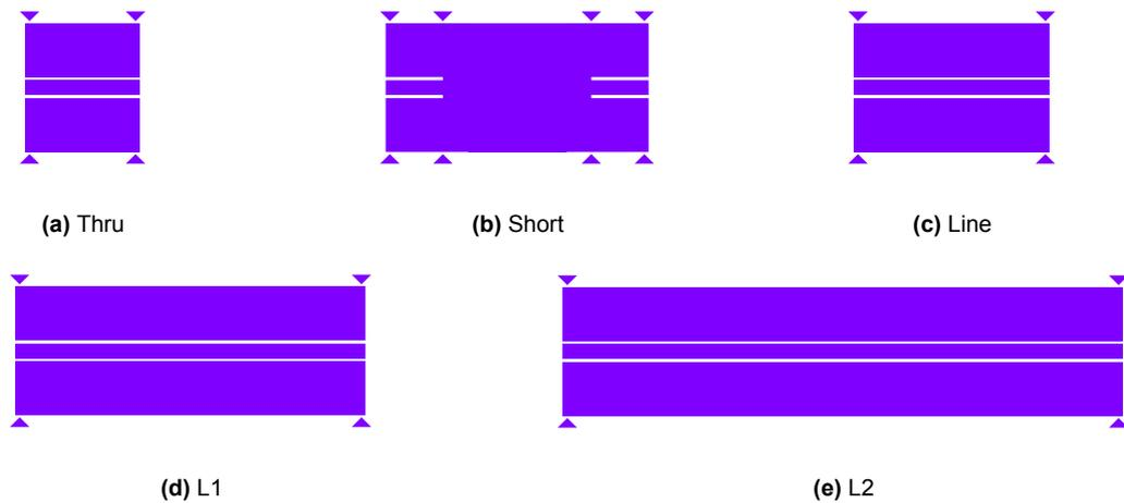
**Figure 5.1:** Features measured during the preliminary TRL measurements. Indigo indicates aluminum.
