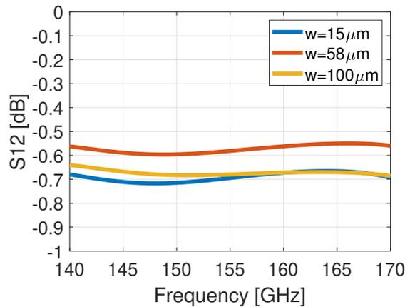
**Figure 2.19:** Optimization of  $w$  of the microstrip to CPW transition for probe landing: S12.
