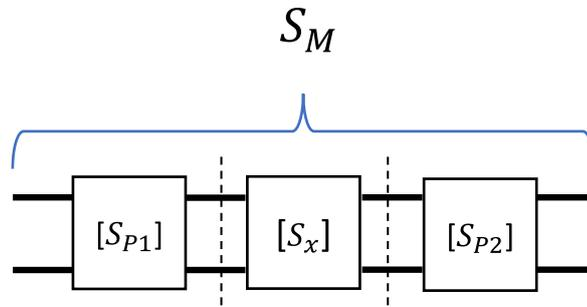
Figure 3.3: Schematic of a measured DUT structure
