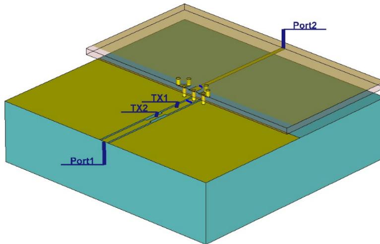
**Figure 4.5:** 3D model of the flip-chip interconnection to the MMICs using CPW transmission lines on the fused silica including a compensation series transmission line.
