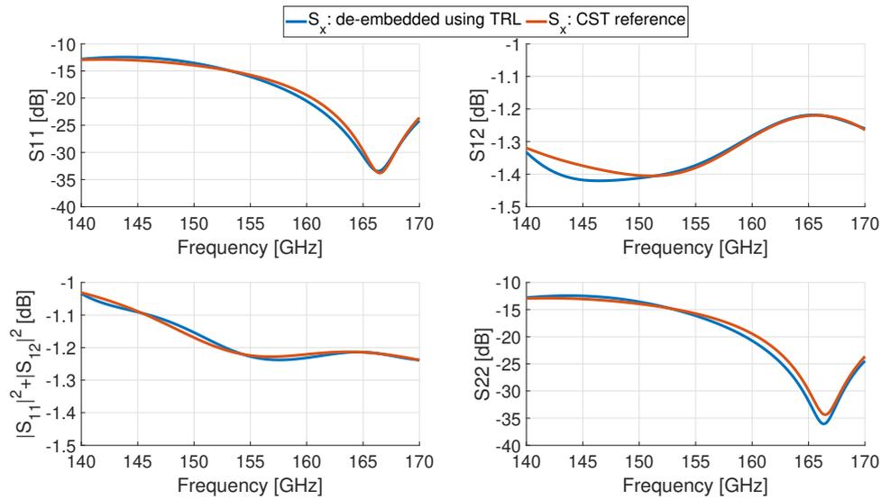
**Figure 3.7:** Comparison between the de-embedded S-parameters in between the error boxes using TRL1 vs CST reference simulation
