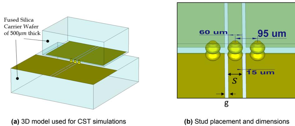
**Figure 2.1:** Flip-Chip interconnection using CPW transmission lines.
