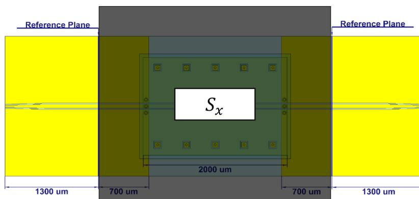
**Figure 3.6:** Back-to-back test structure with the de-embedded subpart indicated in black
