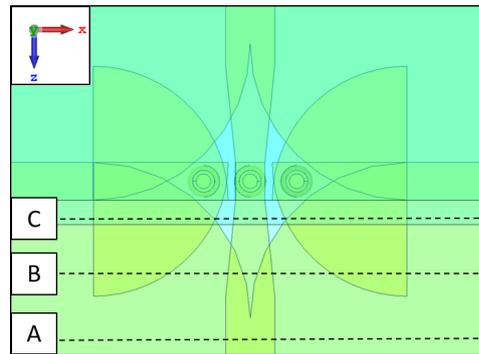
**Figure 2.12:** Top view ( $xz$ -plane) of the via-less Flip-Chip microstrip interconnection, with A, B, and C indicating different  $xy$ -cuts.
