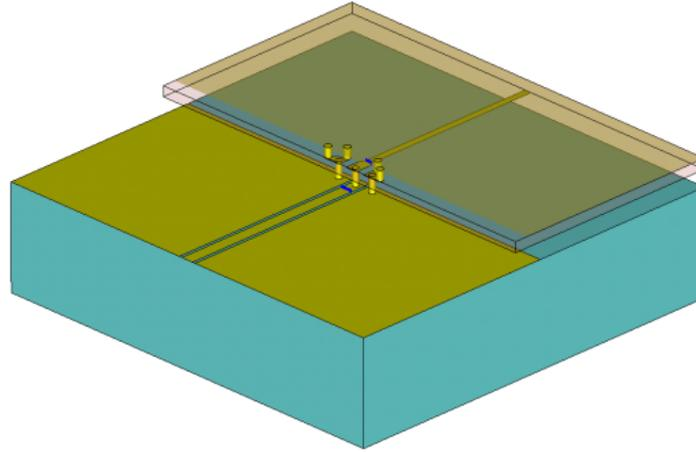
**Figure 4.1:** 3D model of the flip-chip interconnection to the MMICs using CPW transmission lines on the fused silica and representing the studs by cylinders with a radius of  $30\ \mu\text{m}$ . The blue lines indicate the reference planes used for de-embedding the S-parameters of the interconnection.
