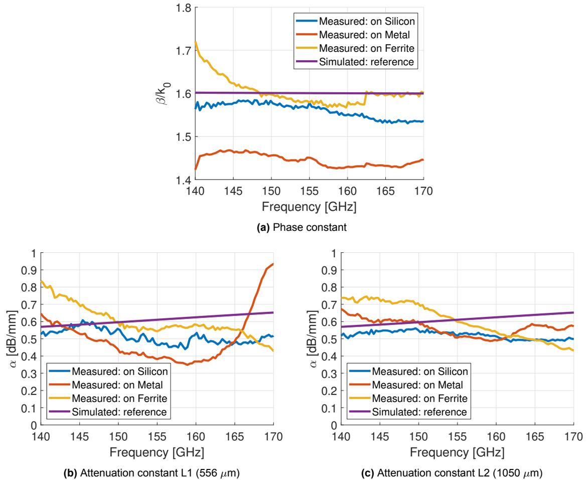
**Figure 5.4:** Propagation constant obtained from measurement using TRL1, compared to a reference CST simulation of the same line on semi-infinite fused silica.
