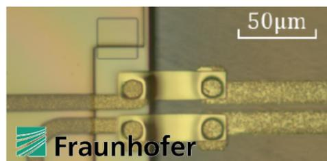
(c) Beam-lead bonding [6]
