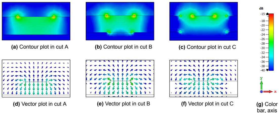
**Figure 2.13:** 2D Electric field relative to the maximum in  $xy$ -cuts A, B, and C, as indicated in Fig. 2.12.
