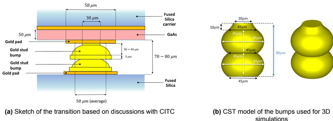
**Figure 1.5:** Physical model of the two Au stud bumps placed on top of each other
