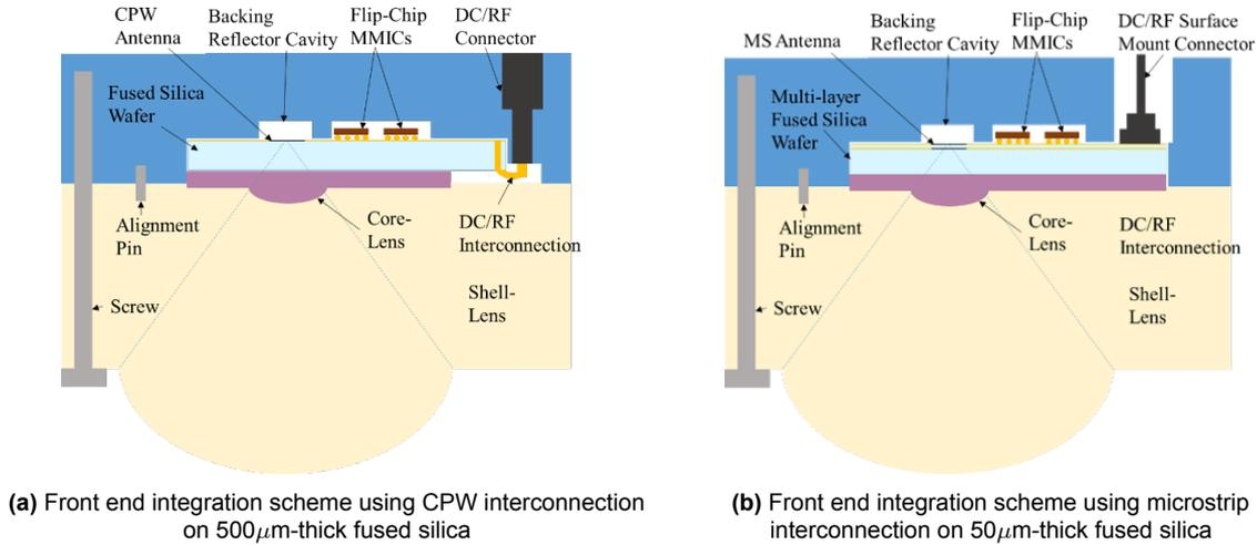
Figure 1.7: Front end integration between MMICs and antenna
