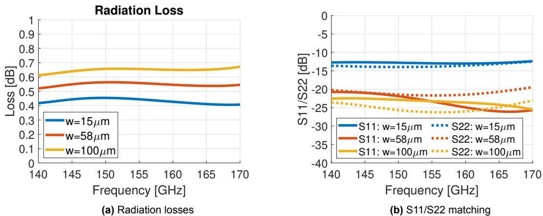
**Figure 2.20:** Optimization of  $w$  of the microstrip to CPW transition for probe landing.
