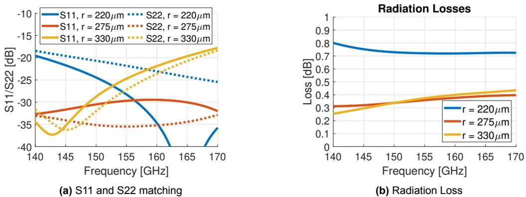
Figure 2.9: Simulated performance of via-less flip-chip microstrip interconnection for varying quarter-circle radius  $r$  of  $220 \mu\text{m}$ ,  $275 \mu\text{m}$ , and  $330 \mu\text{m}$ .
