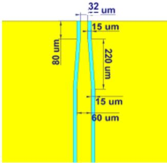
Figure 2.16: CPW probe landing transition
