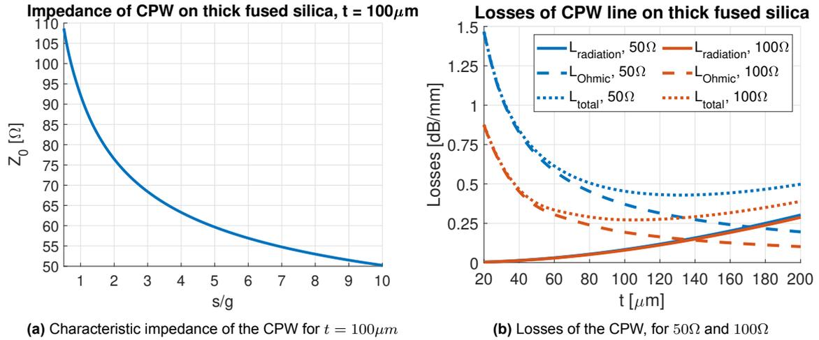
**Figure 1.9:** Characteristic impedance and losses of a CPW transmission line on thick fused silica dielectric, found using the TL Tool [23]
