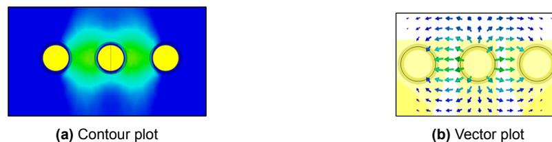
**Figure 2.14:** 2D Electric field relative to the maximum in the  $xy$ -plane of the studs for  $y = d/2$ , where  $d$  is the separation between the two transmission lines or the total height of the studs.
