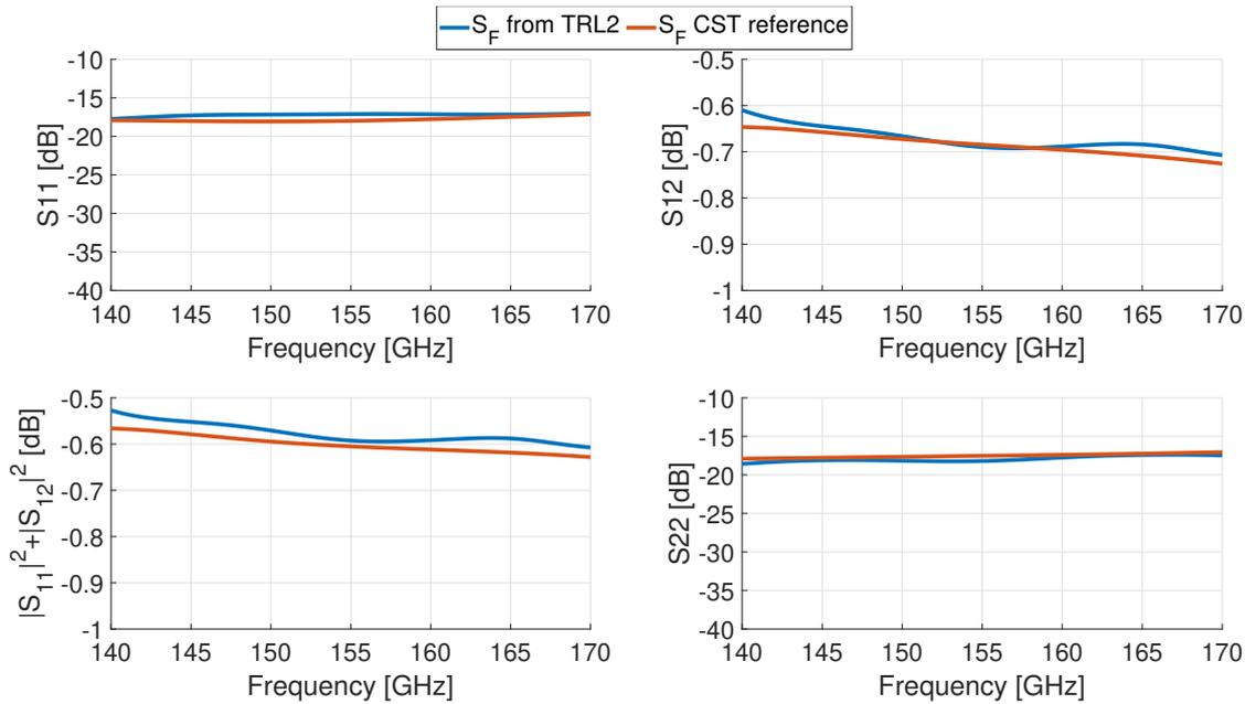
**Figure 3.11:** Comparison between the resulting  $S_F$  found from simulation of the TRL2 back-to-back test structures and the TRL2 MATLAB code vs CST reference simulation.
