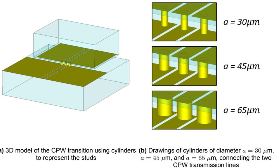
**Figure 2.4:** 3D models of the flip-chip CPW interconnection for varying cylindrical studs.
