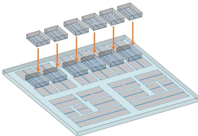
**Figure 3.13:** Illustration of the flip-chip process for the fabricated features included in the mask
