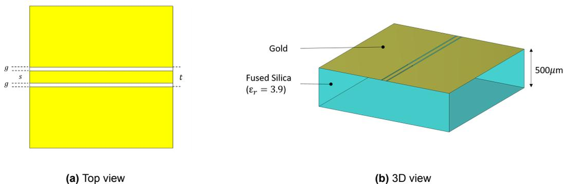
Figure 1.8: Coplanar waveguide (CPW) transmission line on 500  $\mu\text{m}$  thick fused silica
