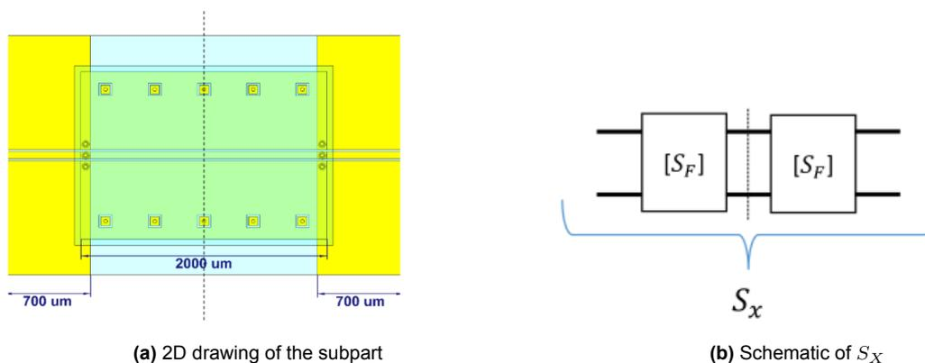
**Figure 3.8:** Subpart of back-to-back CPW test structure corresponding to  $S_X$
