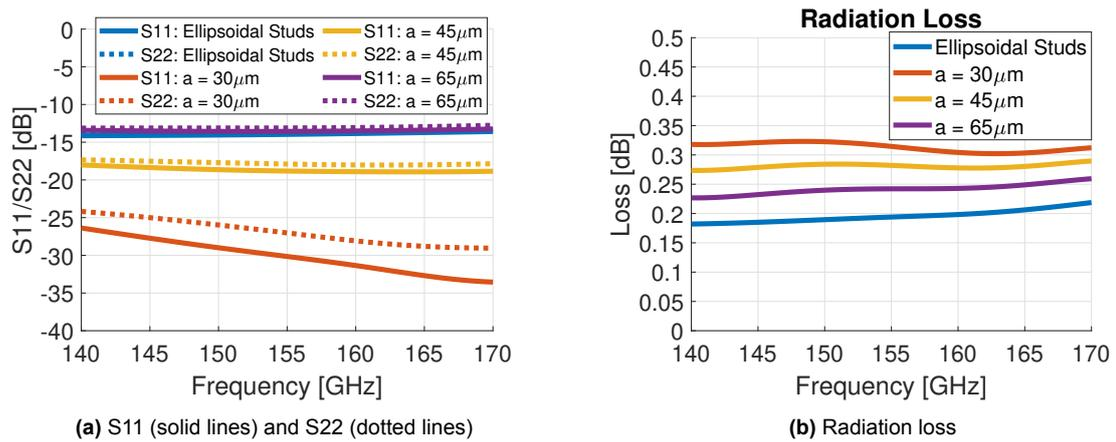
**Figure 2.5:** Results from full-wave simulations of the flip-chip CPW interconnection using cylindrical studs from Fig. 2.4, and ellipsoidal studs from Fig. 1.6b.
