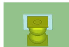
(c) Flip-chip stud for mechanical support
