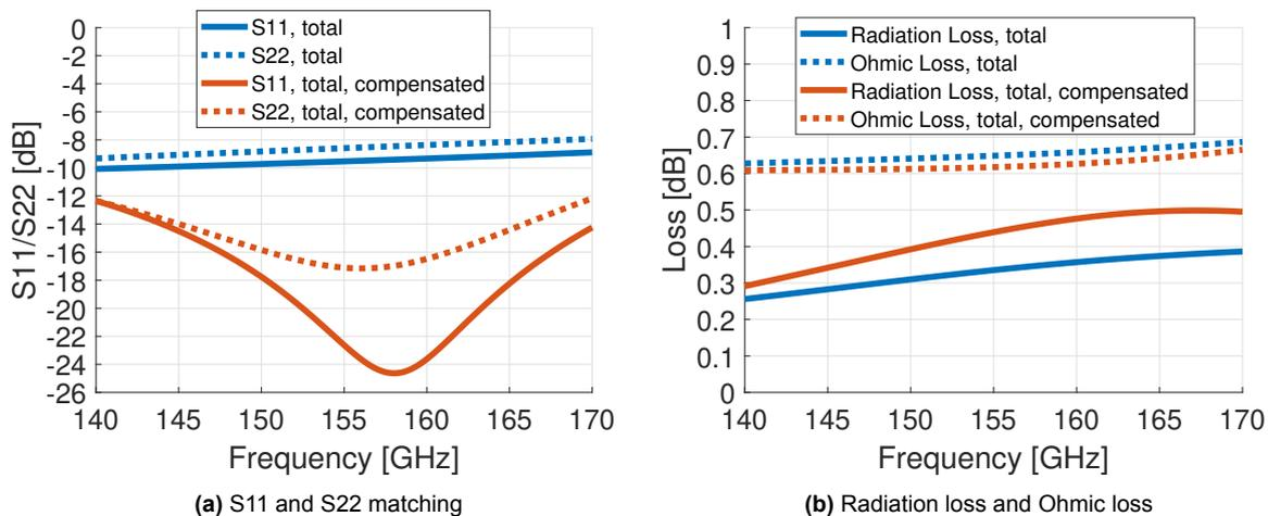
**Figure 4.6:** Comparison of the simulated performance in CST between the flip-chip CPW interconnection to the MMICs from Fig. 4.1 and the interconnection including the high impedance section compensation from Fig. 4.5.
