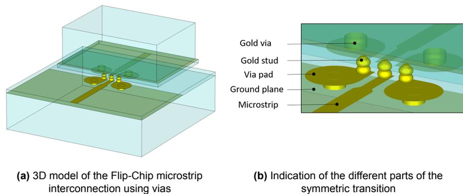
**Figure 2.6:** 3D models of the flip-chip microstrip interconnection using vias.
