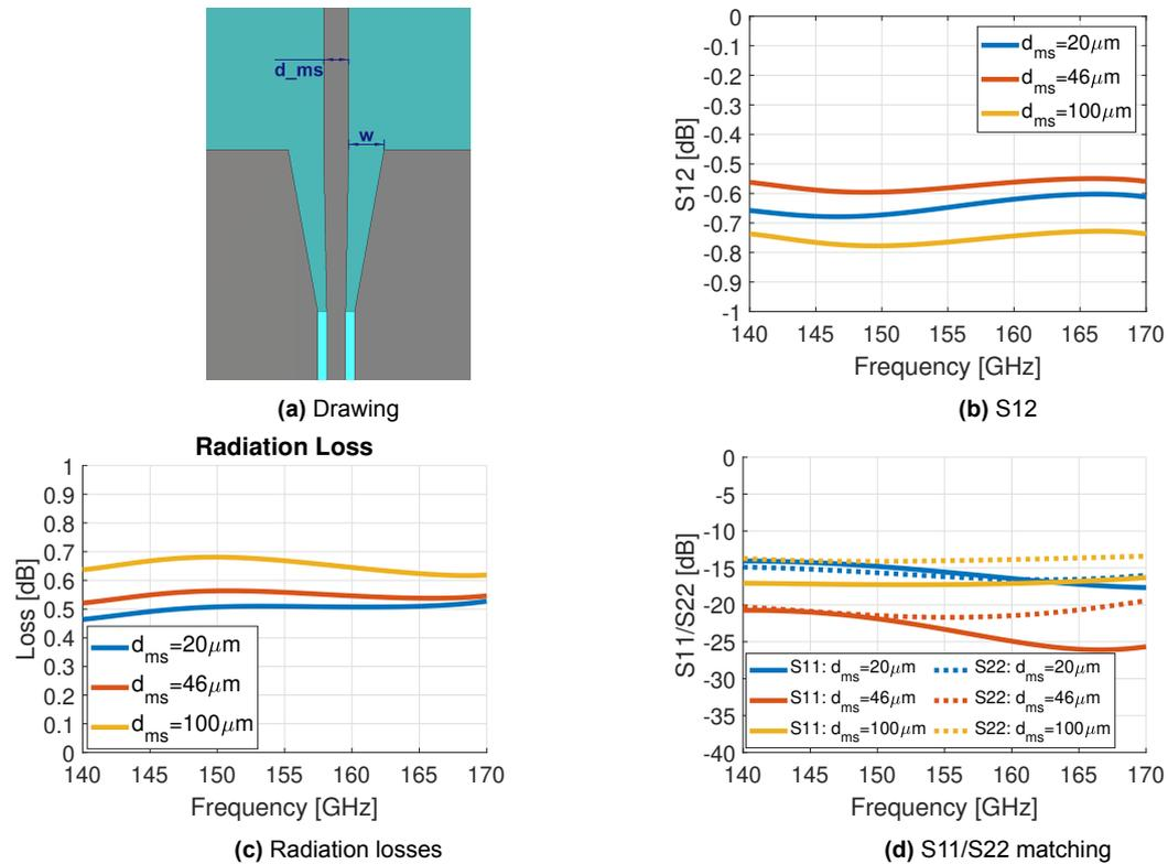
Figure 2.18: Optimization of  $d_{ms}$  of the microstrip to CPW transition for probe landing.
