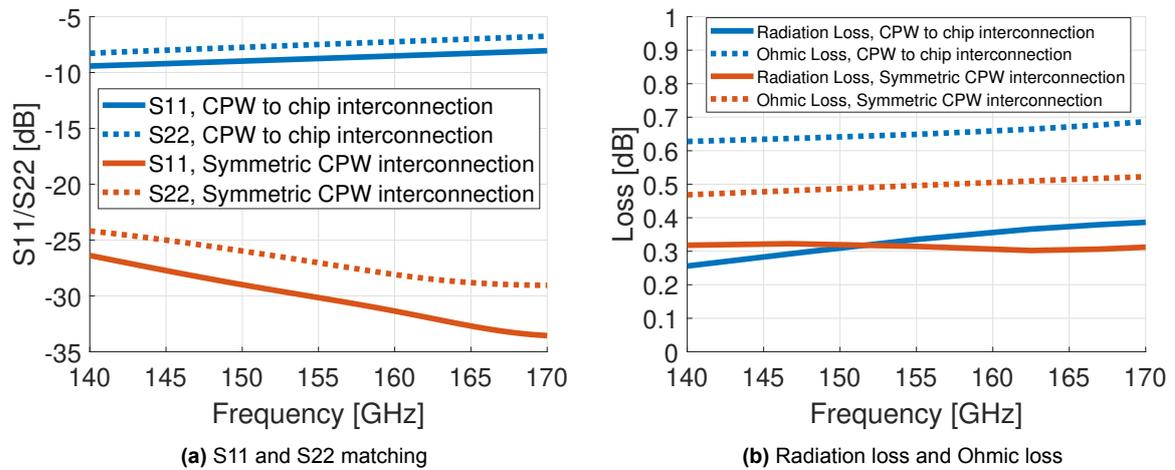
**Figure 4.2:** Comparison of the simulated performance in CST between the flip-chip CPW interconnection to the MMICs from Fig. 4.1 and the symmetric CPW interconnection from Fig. 2.4a for cylinder diameter of  $30\ \mu\text{m}$ .
