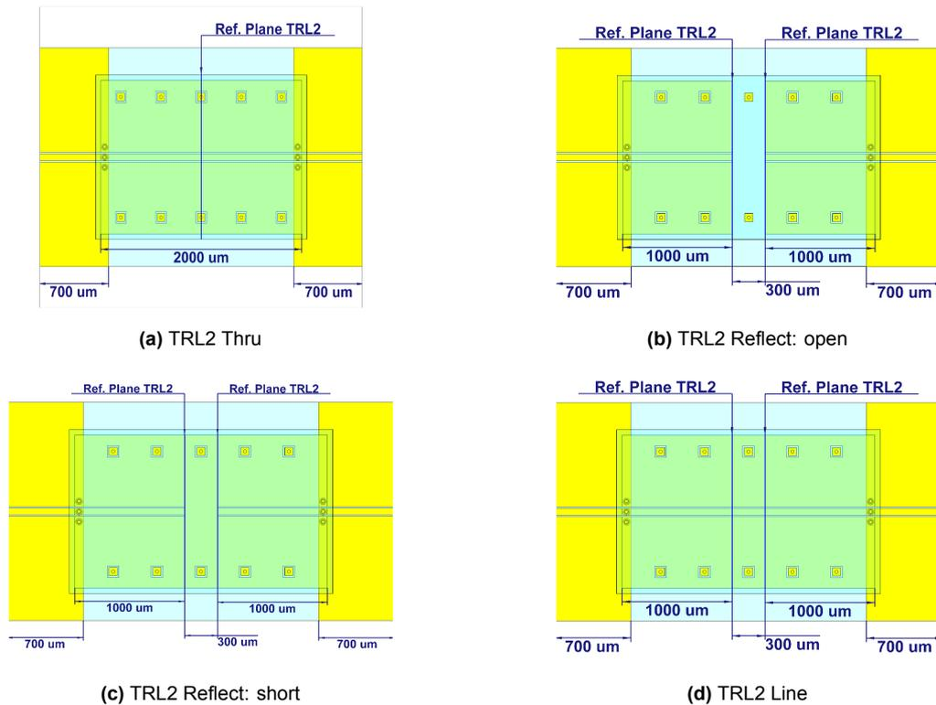
Figure 3.9: 2D models of the TRL2 structures.
