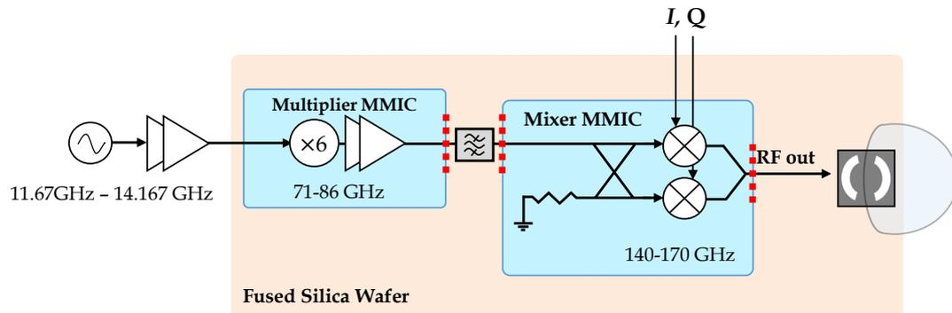
**Figure 1.4:** Circuit diagram of the MMIC integration. The red dotted lines indicate the locations of the interconnections.
