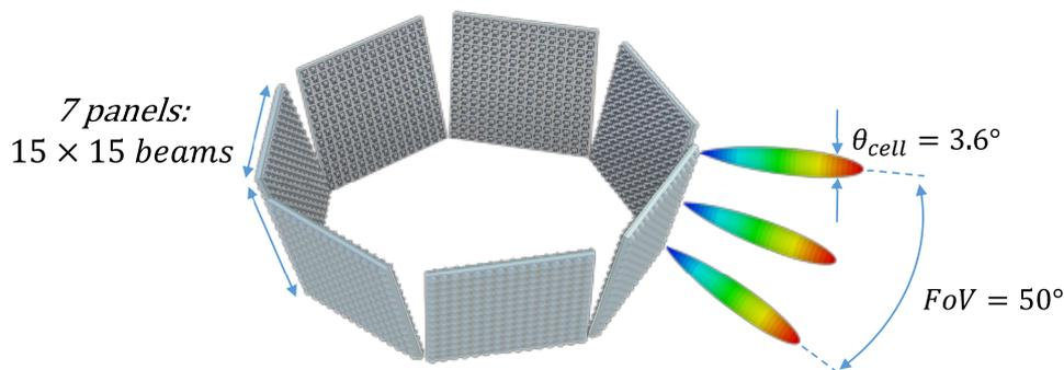
**Figure 1.2:** Sketch exemplifying the multi-beam base station synthesis for the link demo using  $N$  lens array panels. The example shows  $M=7$  panels with a  $16 \times 16$  lens array per panel ( $N=256$ ).
