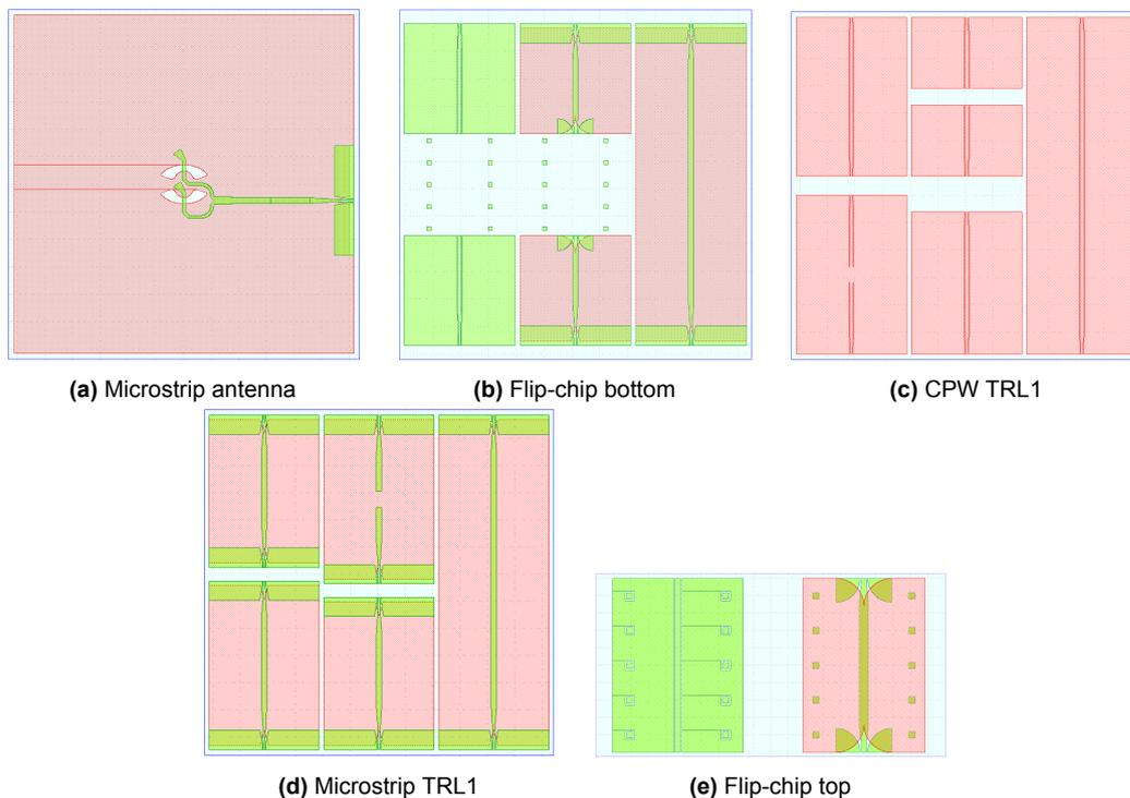
**Figure 3.14:** Mask designs on the 50 $\mu\text{m}$ -thick fused silica wafer.
