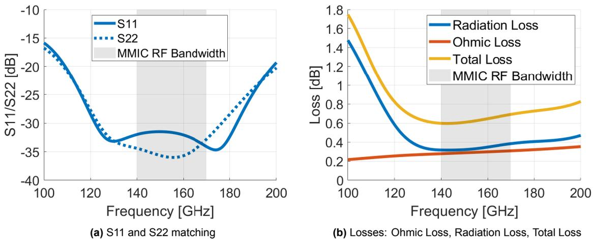
**Figure 2.11:** Simulated performance of via-less flip-chip microstrip interconnection. The frequency range is extended to 100-200 GHz to demonstrate the limited bandwidth.
