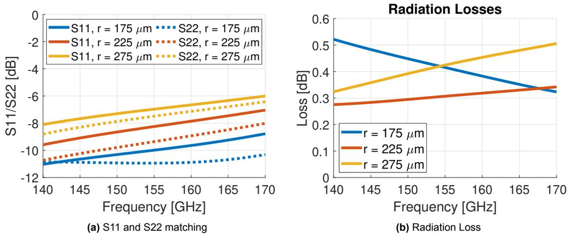
**Figure 4.8:** Simulated performance (from full-wave CST simulation) of the via-less flip-chip microstrip interconnection to the MMIC for varying quarter-circle radius  $r$  of  $175 \mu\text{m}$ ,  $225 \mu\text{m}$ , and  $275 \mu\text{m}$ .
