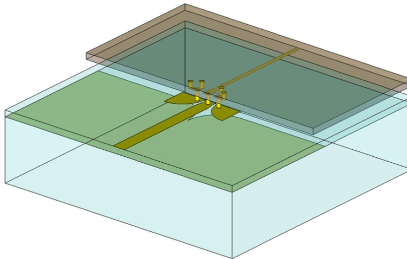
**Figure 4.7:** 3D model of the flip-chip interconnection to the MMICs using microstrip transmission lines on the fused silica.
