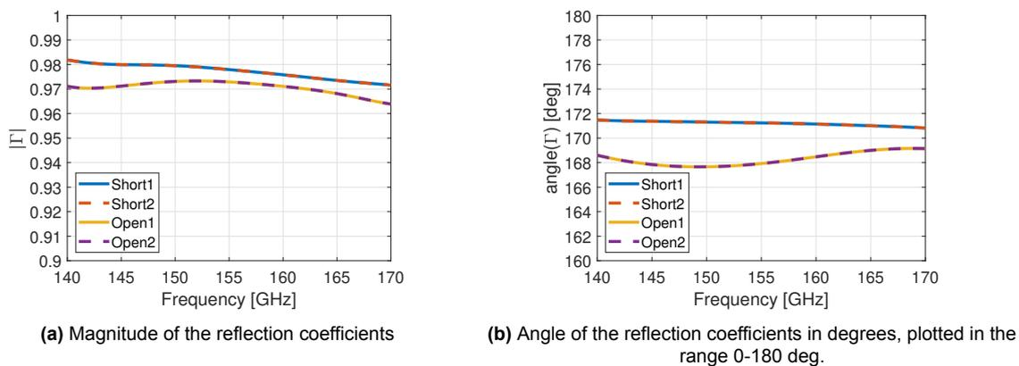
**Figure 3.5:** Reflection coefficient results obtained using the TRL for both Reflect: short and Reflect: open. 1 and 2 as indicated in Fig. 3.2b. Short1 and open1 are the  $\Gamma_1$  (reflection coefficient at port 1) for the short and open circuit, whereas short2 and open2 are the  $\Gamma_2$  (reflection coefficient at port 2) for the short and open circuit.
