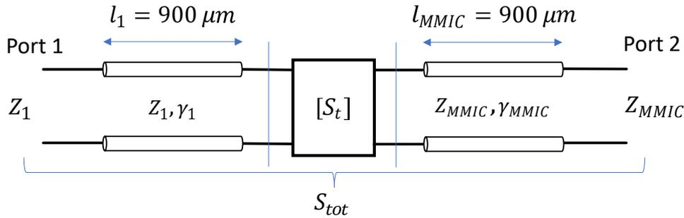
**Figure 4.3:** Schematic of the simulated flip-chip CPW interconnection to the MMICs. The transmission lines on both sides are de-embedded to obtain the S-parameters of the transition  $S_t$ .
