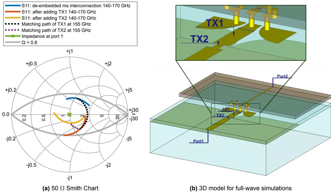
**Figure 4.9:** Flip-chip interconnection to the MMICs using microstrip transmission lines on the fused silica including a compensation series transmission line.
