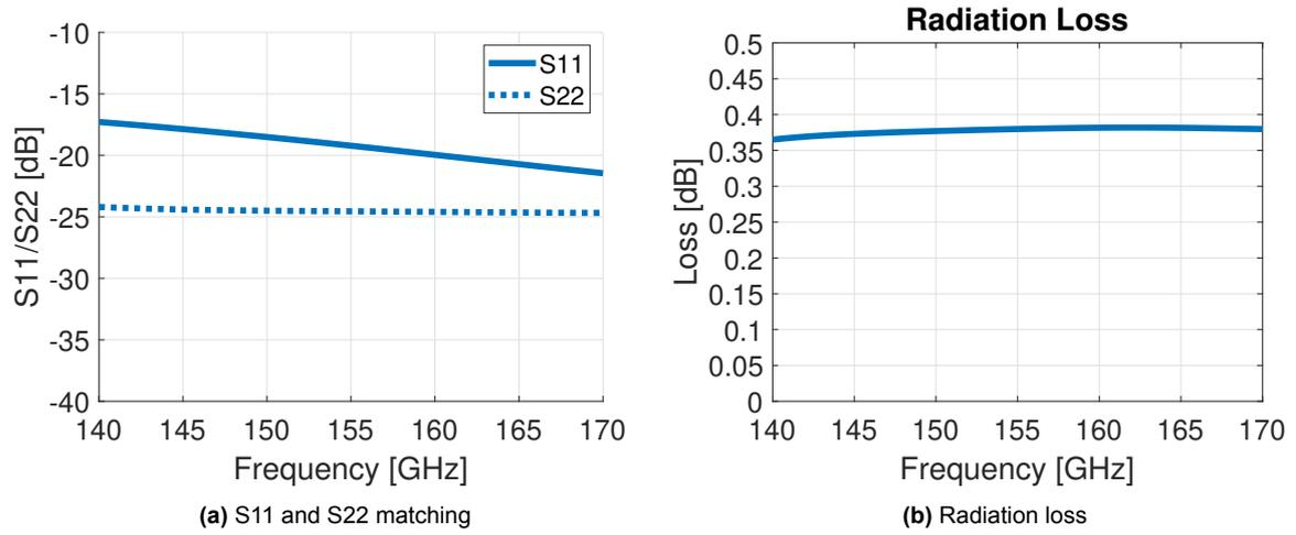
**Figure 2.21:** S11/S22 matching and radiation loss of the microstrip probe landing transition
