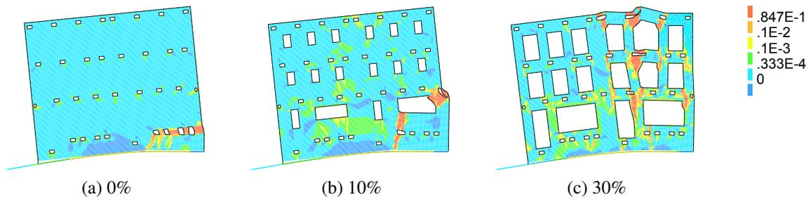
FIG. 4: Maximum principal strain distribution and deformed configuration at 11.5 mm of applied displacement, for different values of opening percentage  $x_1$ : analyses 1, 2 and reference case (see Tab. 2).
