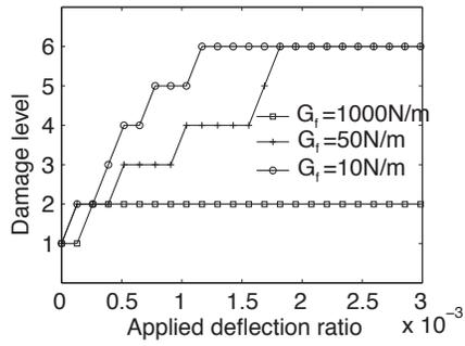
(a) Variation of fracture energy  $G_f$ : analyses 4, 3 and reference case
