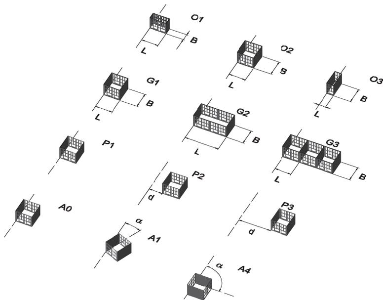
FIG. 2: Overview of the parameters that were varied in the 3D sensitivity study: orientation O, grouping G, position P and alignment A.
