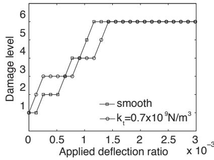
(e) Variation of interface shear behaviour in hogging area: reference case and analysis 11
