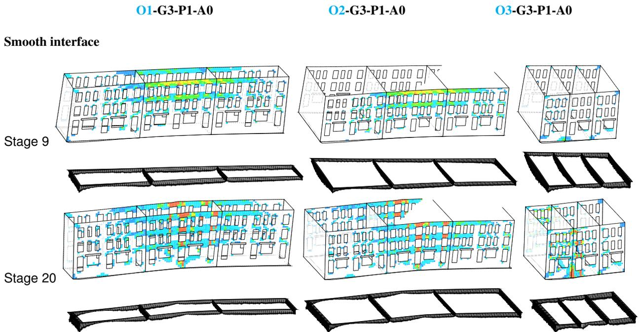
FIG. 6: Crack strain distribution, deformed configuration and soil–structure interface normal stresses: orientation variation for the G3-P1-A0 cases. In Stage 9 the tunnel boring machine passes the building. In stage 20 the machine is fully passed.
