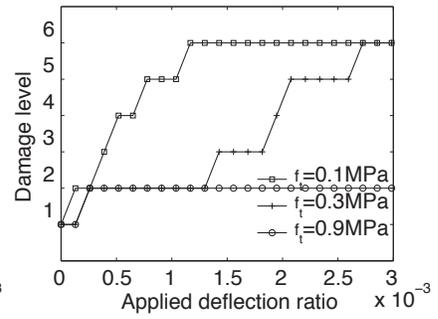
(c) Variation of tensile strength  $f_t$ : reference case and analyses 7 and 8
