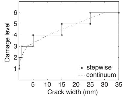
FIG. 11: Maximum crack width vs damage level: step (Tab. 4) and continuous functions.
