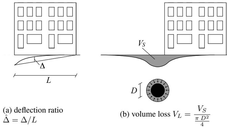
FIG. 3: Indicators of the applied deformation for the (a) 2D and (b) 3D analyses.
