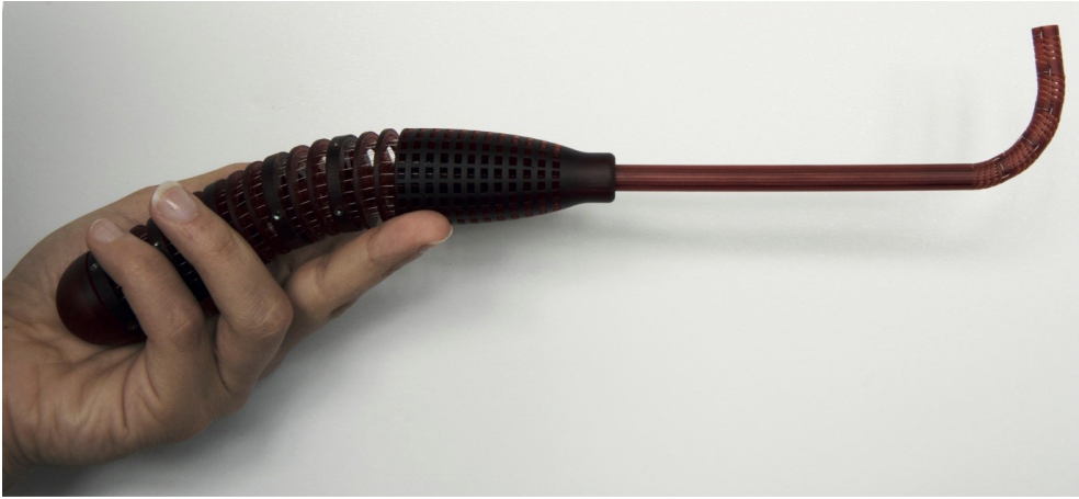
Figure 3.6: The assembled HelicoFlex prototype showing a single curve.
