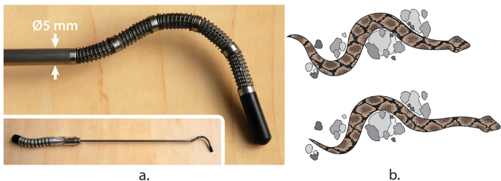
Figure 6.1: Flexible surgical instrument and Follow-the-Leader propagation. (a) The MultiFlex, an \varnothing 5 mm flexible instrument with 10 degrees of freedom [28]. The instrument is controlled by manually adjusting the shape of the handle, which is mimicked by the flexible part of the shaft. (b) Snake moving through a cluttered environment by transferring a curved path initiated by its head along its body. This motion is referred to as a Follow-the-Leader propagation.
