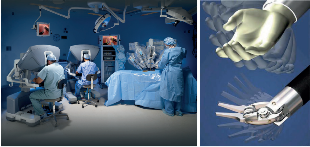
Figure 1.4: Left, the Da Vinci surgical system (Sunnyvale, California, USA, Intuitive Surgical): a robotic master-slave system containing multiple robotic arms that maneuver the instruments, and one or two surgeon consoles. (© 2016, Intuitive Surgical, Inc. (CC BY-SA 3.0, https://creativecommons.org/licenses/by-sa/3.0 ). Right, the steerable instrument called the EndoWrist incorporated in the Da Vinci system. The two degrees of freedom of the joint mimic the maneuverability of a human wrist (adapted from [17]).
