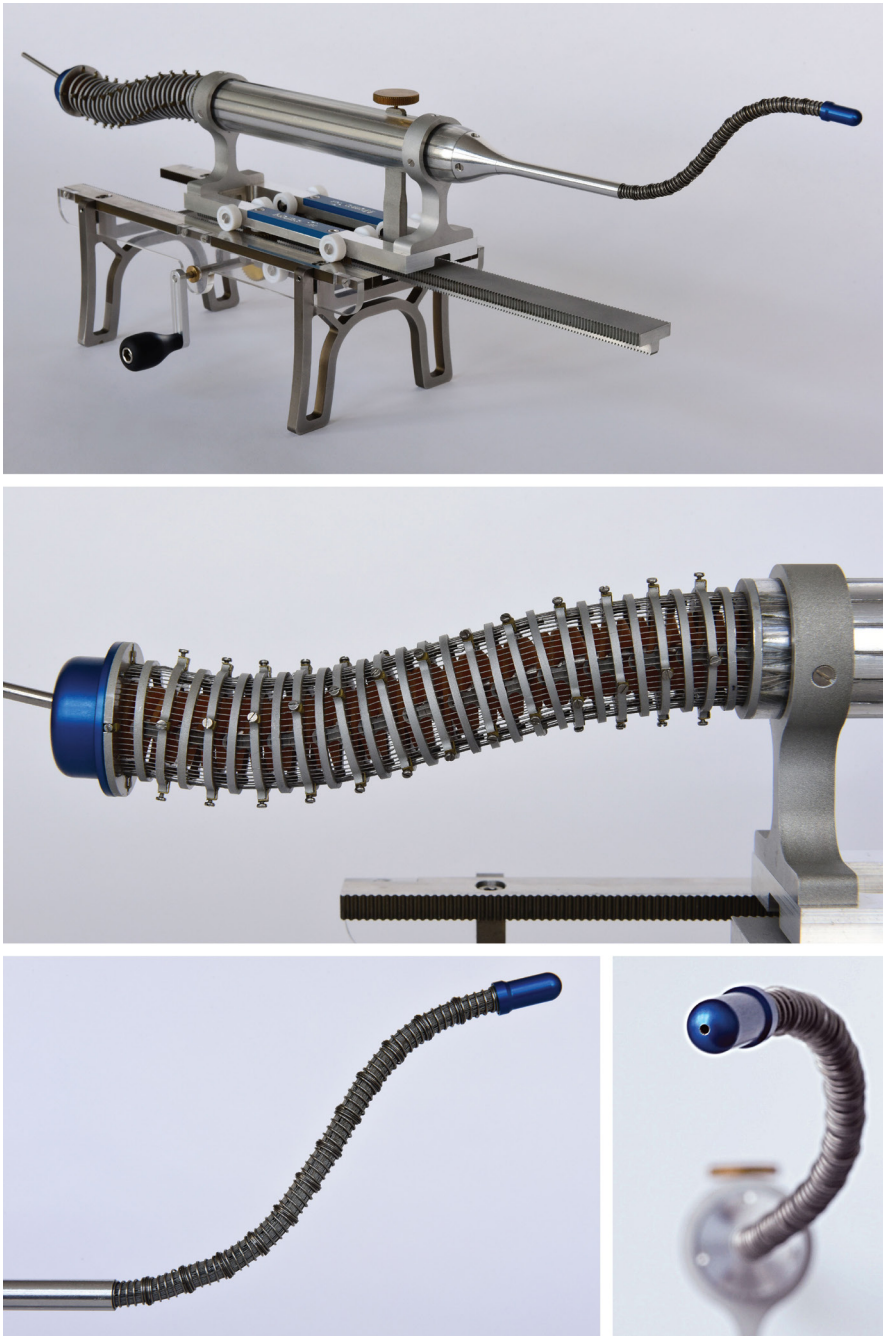
Figure 4.6: Proof of concept prototype; the MemoFlex I. All parts were fabricated out of aluminum, except for the wheels (nylon), gear rack (stainless steel) and gears (brass). The outside of the shaft is transparent to allow visual feedback of the cables during their assembly.
