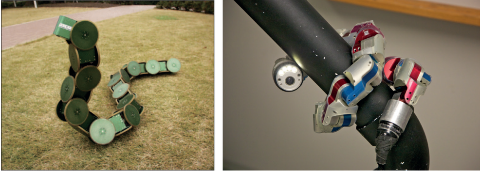
Figure 1.7: Snake-like robots. Left: ACM-R3 snake robot developed at the Tokyo Institute of Technology © [2009] IEEE [22]. Right: Uncle Sam, a snake robot developed at the Robotics Institute of Carnegie Mellon University. 'Snake robot at the Robotics institute'; image by Jiuguang Wang, www.robo.guru , licensed under CC BY-SA 2.0.
