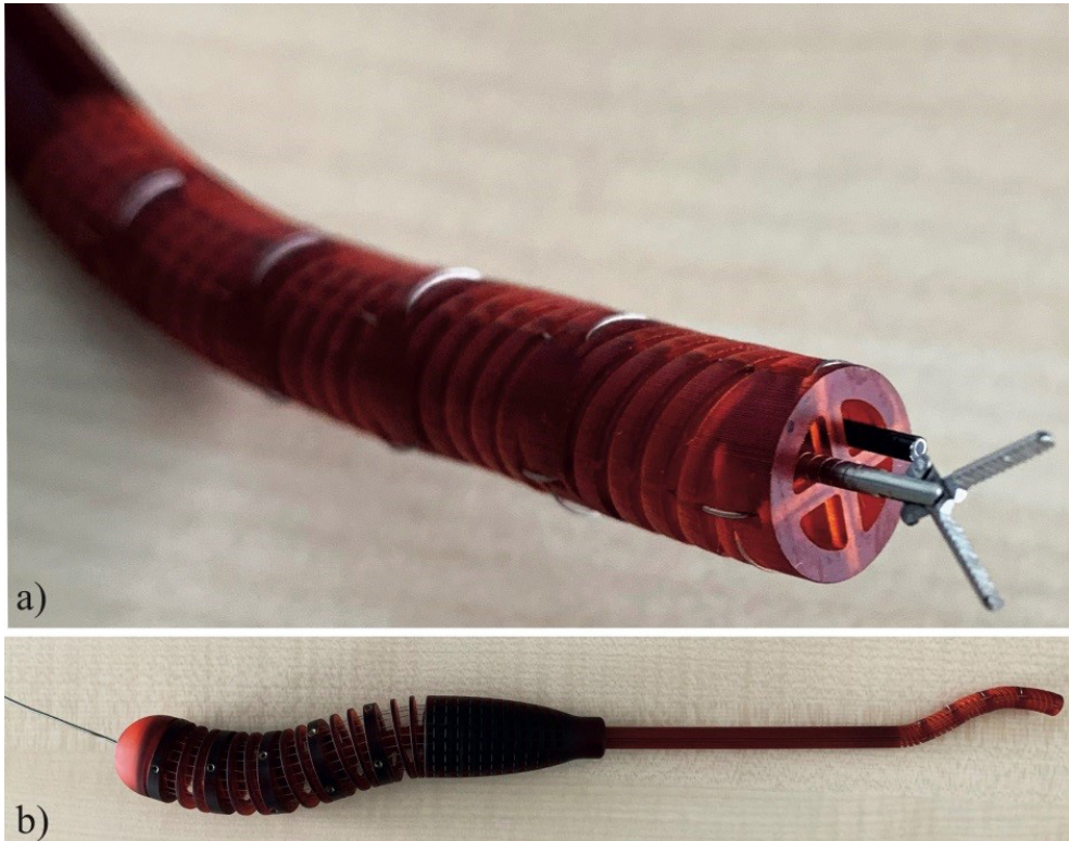
Figure 3.8: Pictures of the HelicoFlex prototype; a) close-up of the compliant shaft of the HelicoFlex with a flexible biopsy forceps in one lumen and a flexible fiber optics endoscope in the second; b) bendable metal rod inserted into one of the lumens to create a certain shape in compliant shaft and keep it in position.
