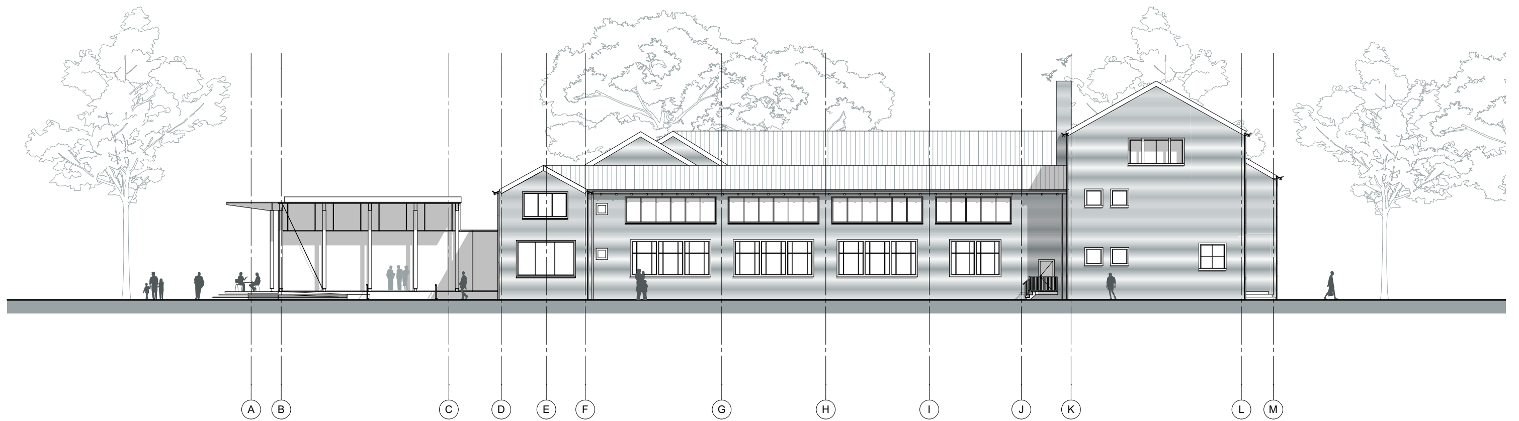
Elevation West Facade 1:250
