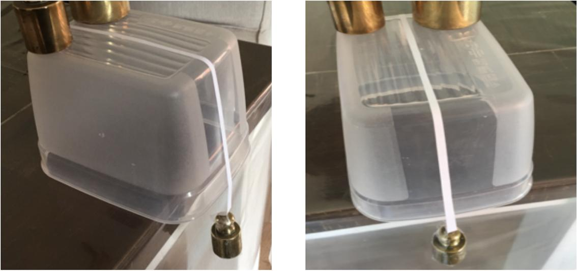
Figure A.2: Proof-of-concept tape pre-tension setup
