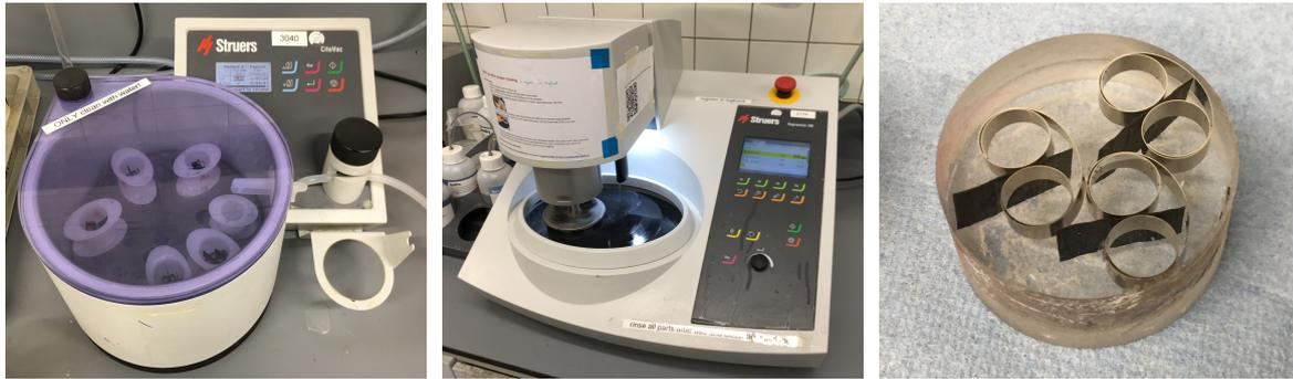
Figure 4.13: Steps taken for cross-sectional epoxy samples preparation. Left: Struers CitoVac, Mid: Struers Tegramin-20 Polishing machine, Right: Cross-sectional sample
