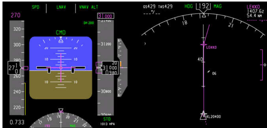
Boeing 747-400 Electronic Flight Instrumentation System as is found in many modern airliners
