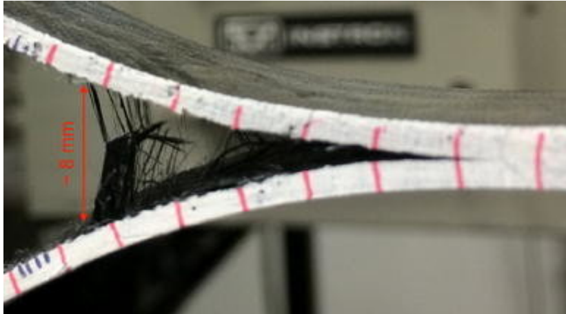
Figure 2.3: Separated-to-intact transition for delaminated composite specimen [10]. Fibers bridging opposite surfaces are observed approaching the crack tip.
