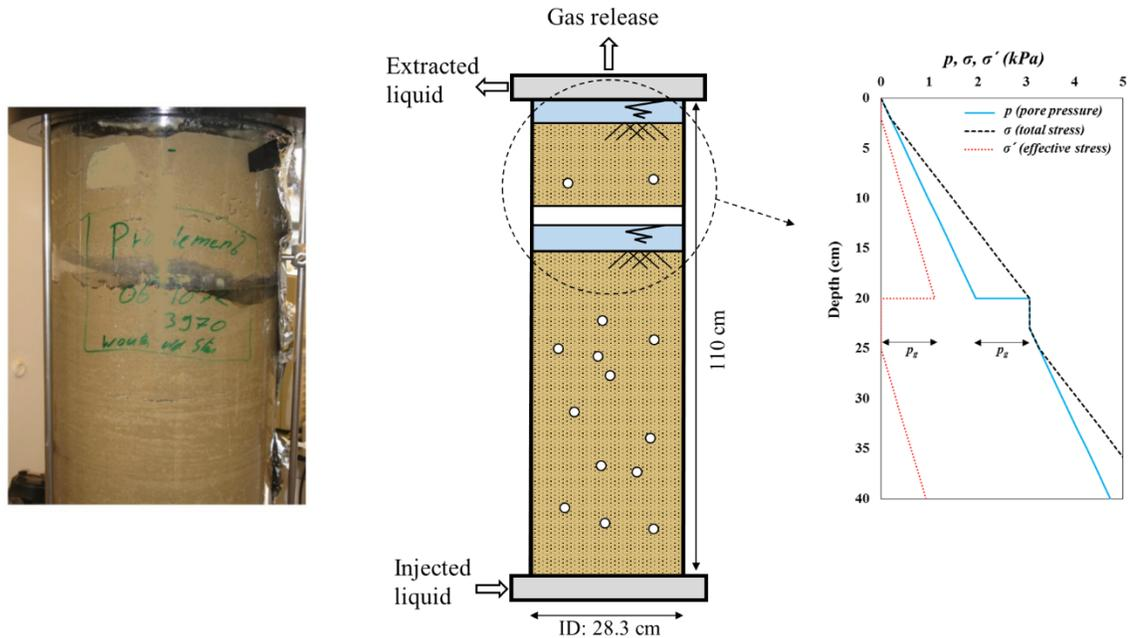
**Figure 4: Occluded gas lenses appeared in the upper part of a sand column, lifting up the overburden, increasing the pore pressure and reducing the effective stress in the underlying soil (Van Paassen, 2009)**
