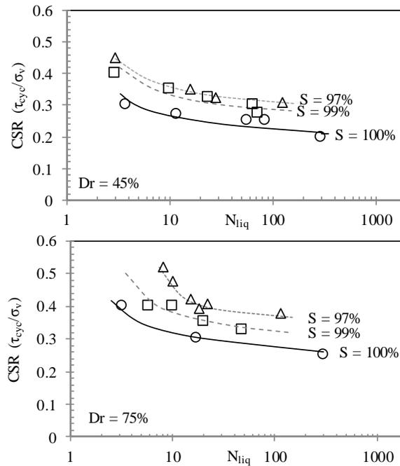
**Figure 3 Response of partially saturated sand under undrained cyclic loading (O'Donnell 2016)**
