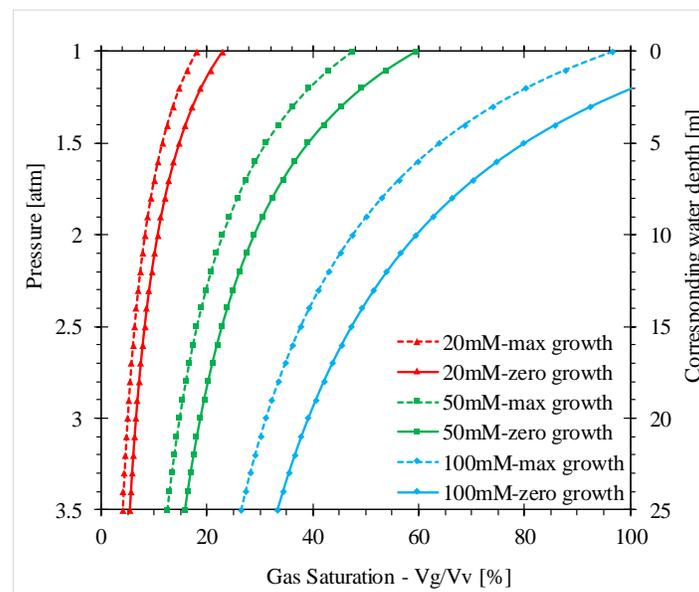
**Figure 1. Gas saturation induced by denitrification as a function of pore pressure for maximal growth (dashed lines) and zero growth (continuous lines) for three different concentrations of consumed  $\text{NO}_3^-$  (from Pham 2017)**
