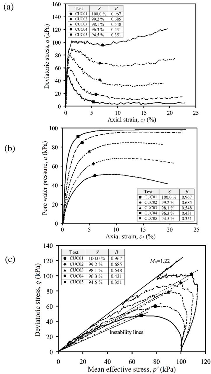
**Figure 2 Mechanical response of a partially saturated sand under undrained monotonic loading. (a) stress-strain response, (b) pore pressure response and (c) effective stress paths (from He and Chu 2014 with permission of ASCE).**
