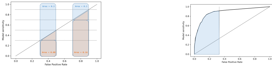
(a) The maximum area underneath an ROC curve between false positive rates 0.7 and 0.9 and between 0.3 and 0.5 is both 0.2, whereas the minimum areas are 0.16 and 0.08, respectively.
