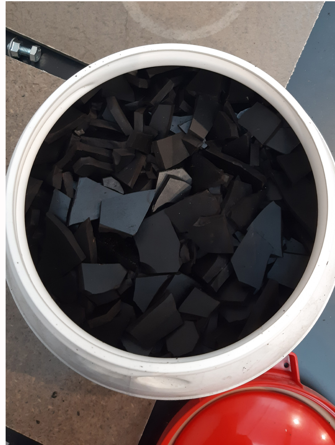
Step 1: Hammering sample plate into small pieces
