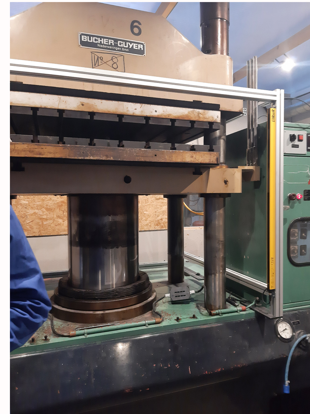
Step 2: Pressing sample plates
