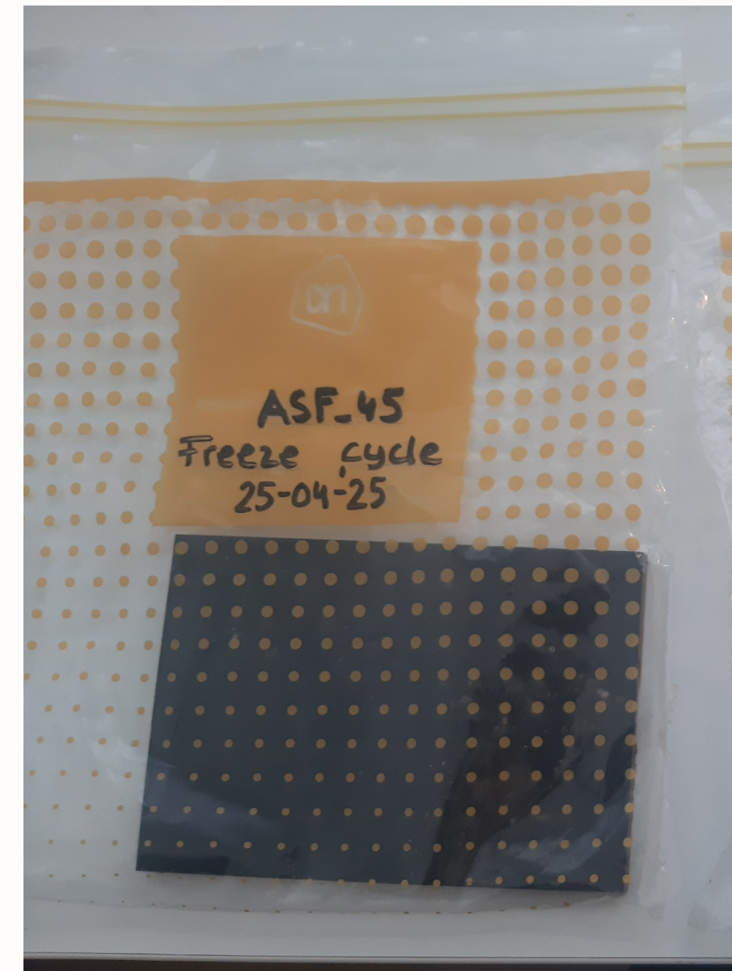
Frost resistance (Time intervals: 8h x 8h x 10 cycles)
