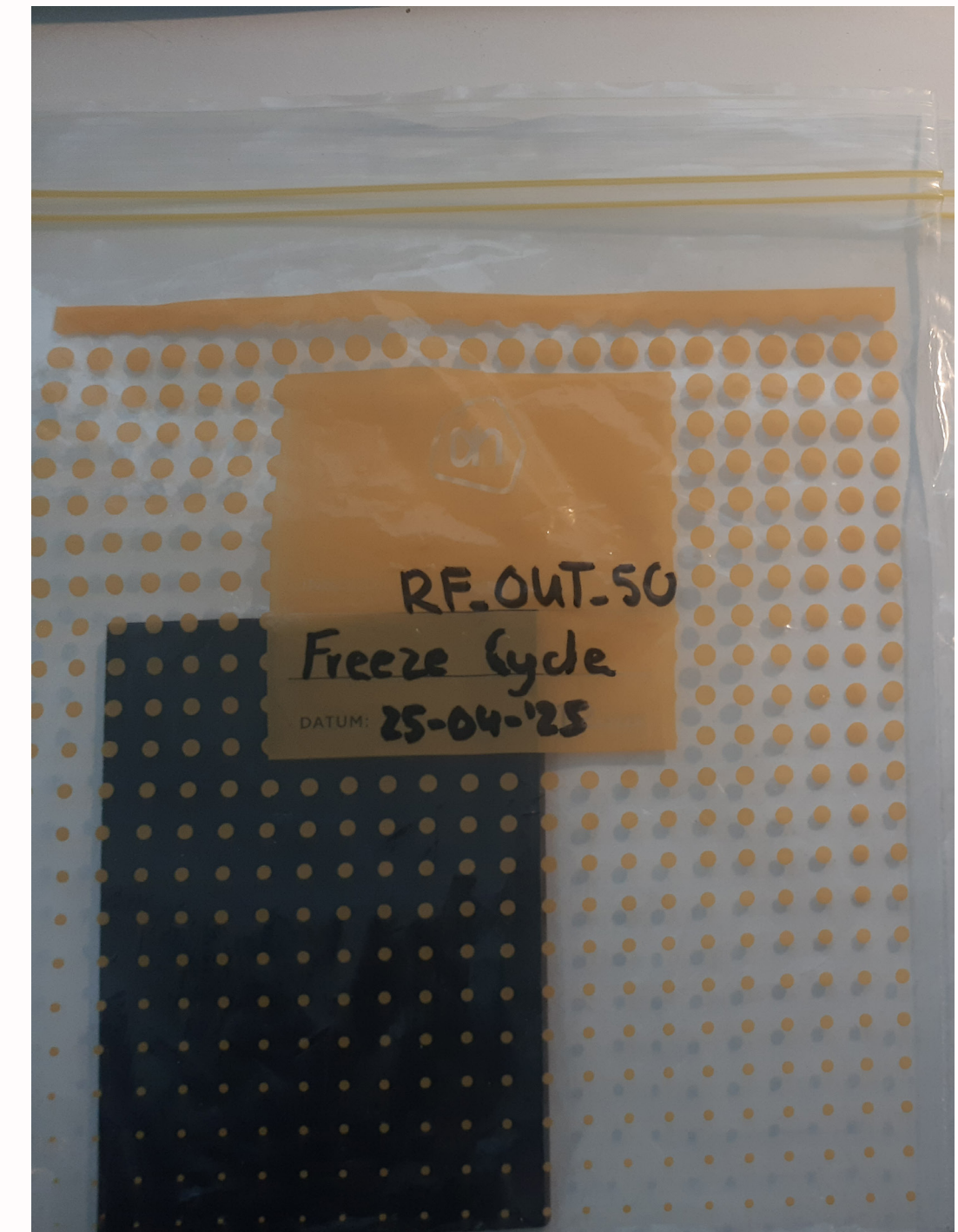
Frost resistance (Time intervals: 8h x 8h x 10 cycles)
