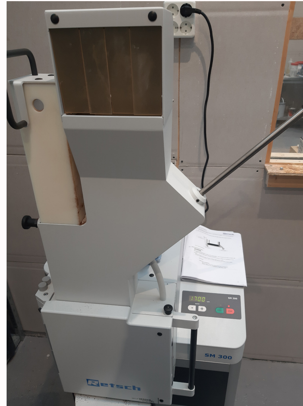
Step 2: Shredding into smaller pieces
