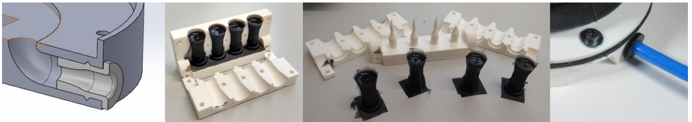
Fig. 2 - Section view of how tube enclosure fits in base plate; mold of the tube enclosure; components retrieved from mold; tube enclosure as assembled in the module
