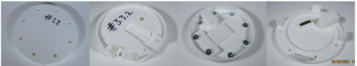
Fig. 6 - Early version of base plate with place for nuts; broken base plate due to broken screw (had to be cut out); first version of shelled base plate; later version of base plate, walls have been removed for easier access to the screws
