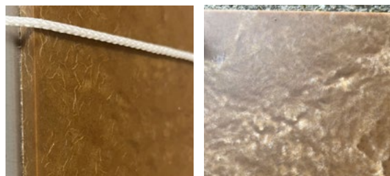
Figure 5.11. Visual comparison of weathered composite surfaces after exposure in the QUV chamber (left) and under in situ weathering conditions (right). The in situ exposure duration corresponds to approximately 3.3 days of accelerated weathering in the QUV chamber.
