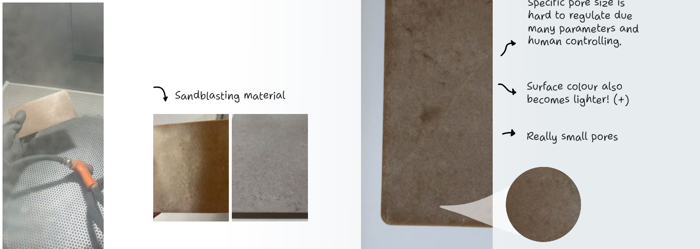
Figure 6.9. Experiment of post-processing surface with abrasive blasting
