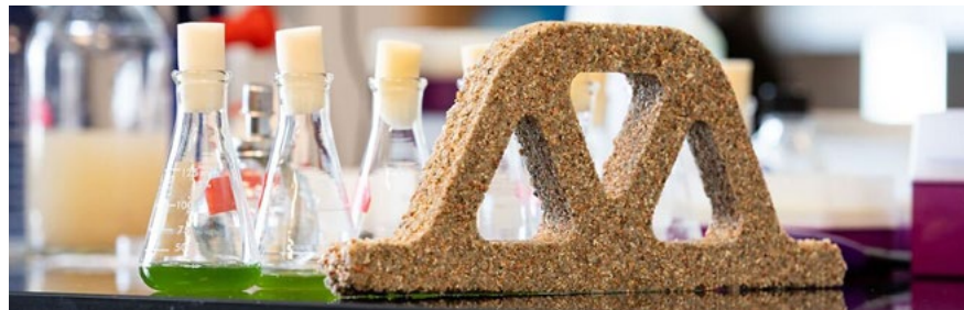
Figure 3.12. Prototype of self-healing brick by university of Colorado Boulder (Source: Self-healing Bricks Eat CO 2 !, 2020)
