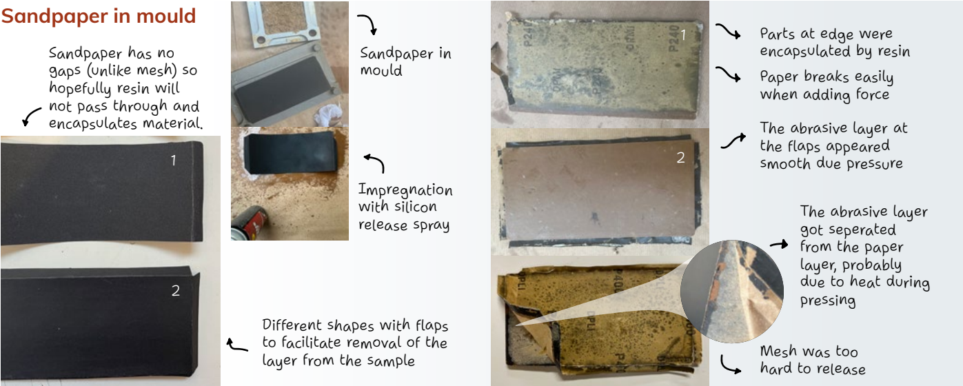
Figure 6.8. Experiments on adding sandpaper in mould
