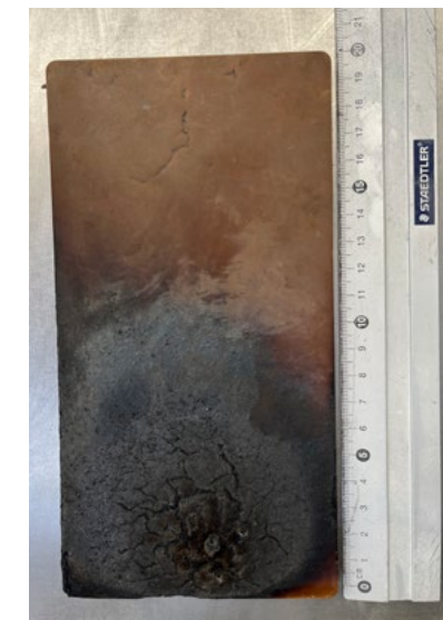
Figure 5.14. Measured flame height is below 150 mm
