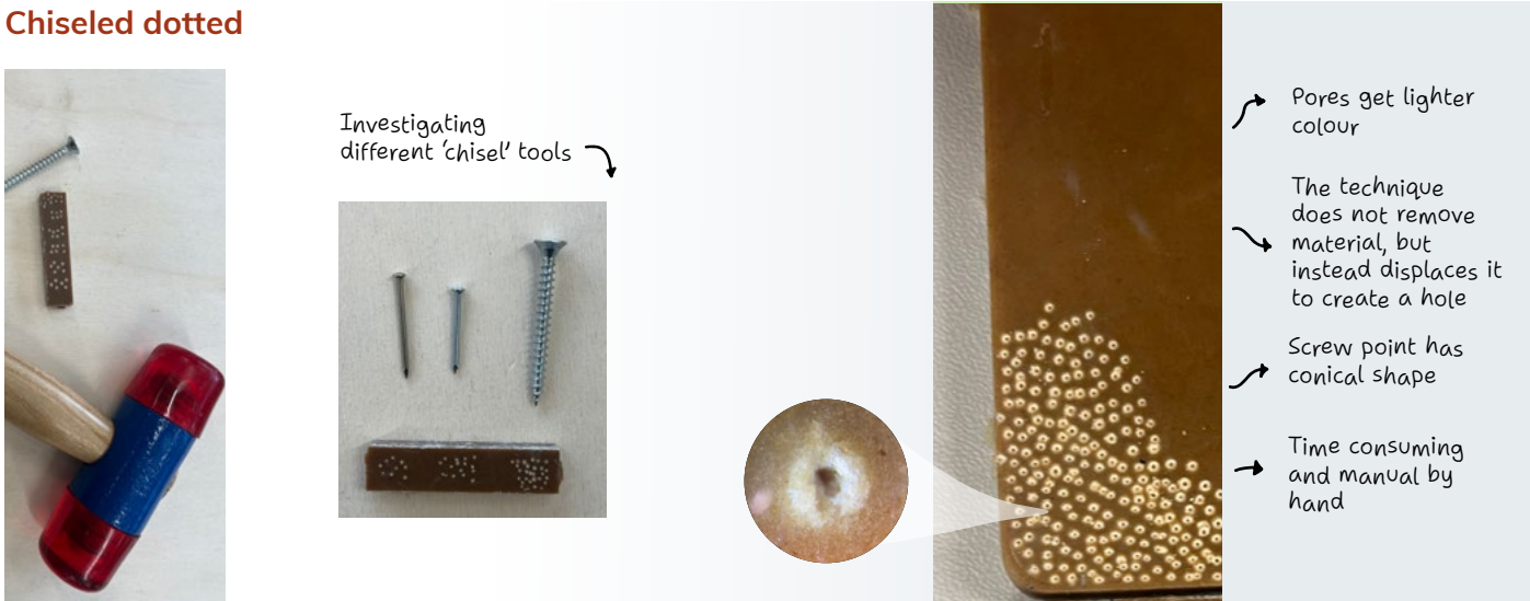
Figure 6.10. Experiment of post-processing surface with manual perforation
