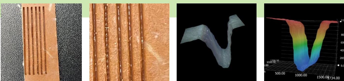
Laser-lined (not final) (multiple depths & diameter 0,4-0,6-0,8)
