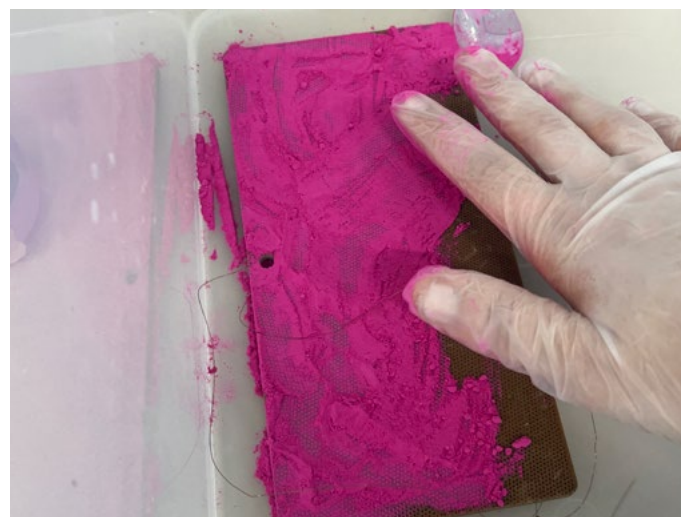
Figure 7.5. Manual particle deposition for particle retention setup
