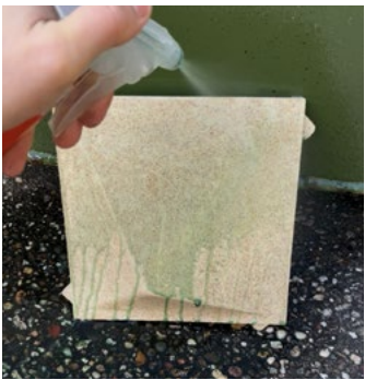
Figure 8.5. Water path analysis using spirulina-coloured water to visualise flow patterns across the selected facade morphology
