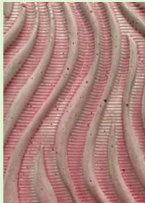
Figure 8.2. Example of a macrostructure which redirects coloured water to certain areas (Source: Mustafa et al., 2021)
