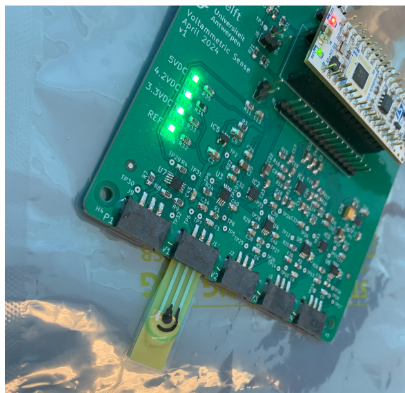
Figure 3.11: Realisation of the prototype running a voltammetry experiment.
