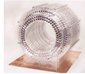
Fig. 2. The (permanent) magnet in Halbach arrays in which the patients are inserted [11].
