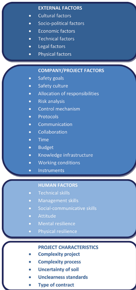
Figure 1. Possible critical factors at macro, meso and micro level and project characteristics (Terwel & Vambersky, 2012).
