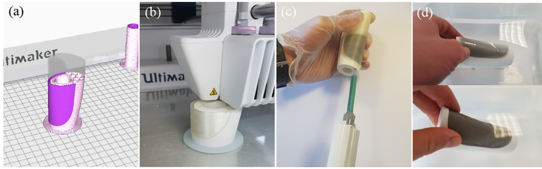
Fig. 1. Hybrid Deposition Manufacturing process used in this paper. (a) Slicing of part in printer software. Hard material is indicated in pink, sacrificial mold part is indicated in purple. (b) Printing of part with sacrificial mold. (c) Low pressure casting of silicone. (d) Curing and demolding.
