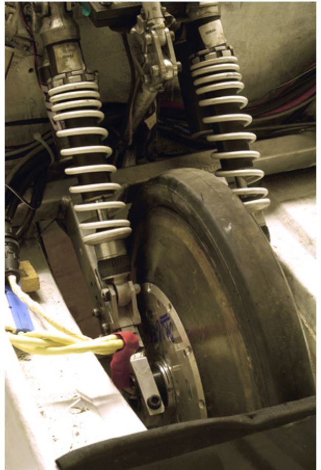
Nuna II is driven by the rear wheel that has an incorporated electric motor.
