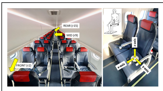
Figure 1. Position of accelerometers in the ATR aircraft and illustration of the basi-centric axes of the human body considered for evaluation of WBV in accordance with ISO2631-1.
