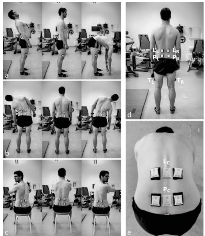
Fig. 2. Illustration of motion sequences, IMU attachment on subject and central IMUs: (a) Flexion/extension (b) Lateral flexion (c) Rotation (d) Attachment of the six IMUs on subject (e) Approximated central orientations, illustrated by central IMUs.
