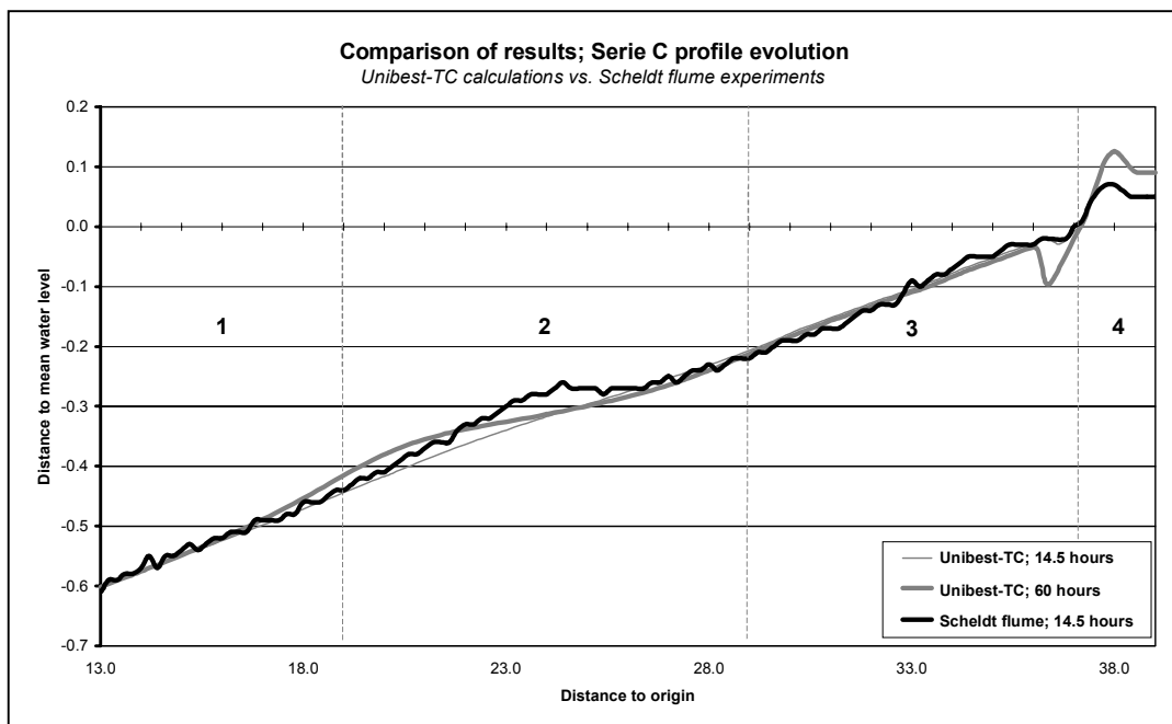
Figure 5-7; Comparing Unibest-TC and Scheldt flume experiments, Series C
