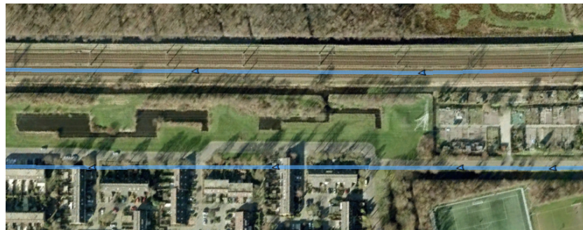
Figure 27: Two segments made on the same railway in different timeframes. Their difference is approx. 80 metres. (Imagery © Aerodata International Surveys and Google (2010).)
