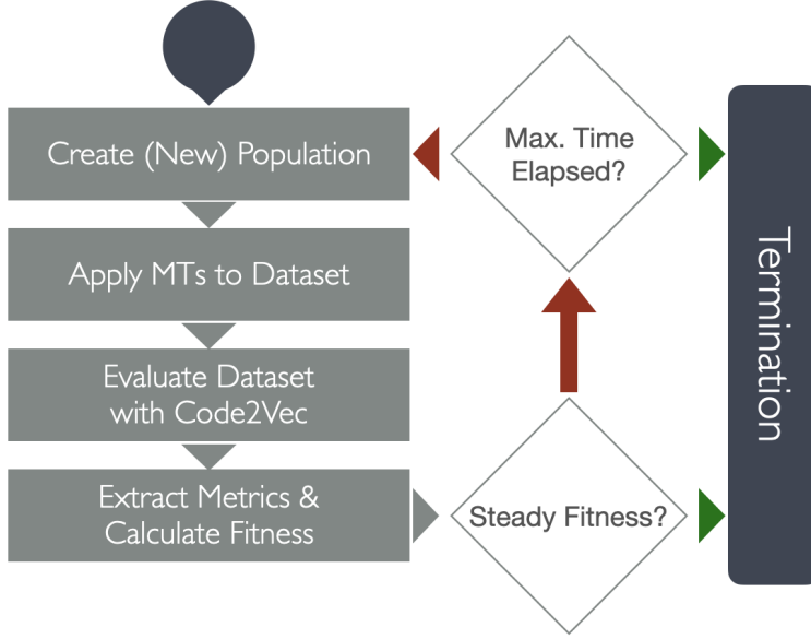
Figure 3.1: schematic Control-Flow of Guided-MT Program
