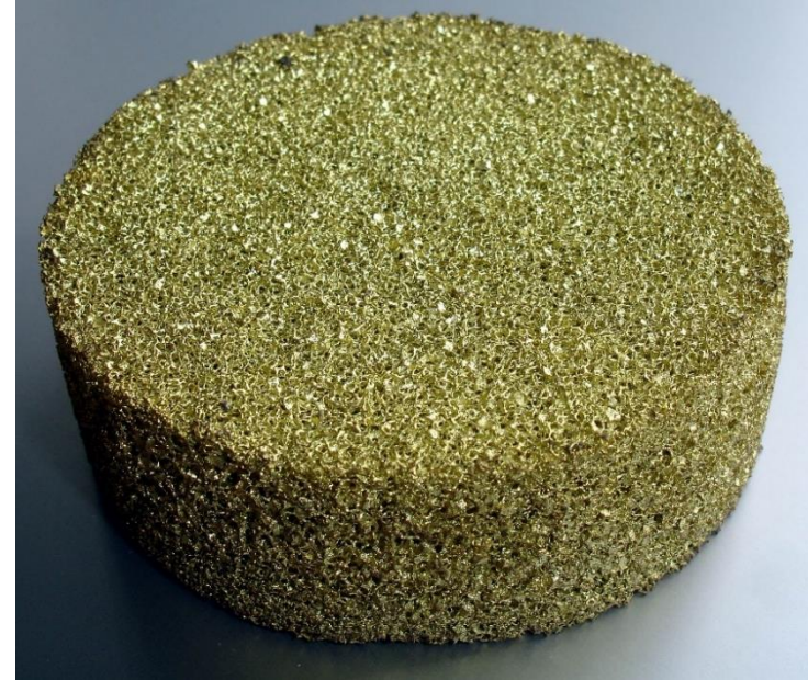
Metallic foam (chemical reaction)
