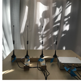
Fig. 7. Uniform linear array setup
