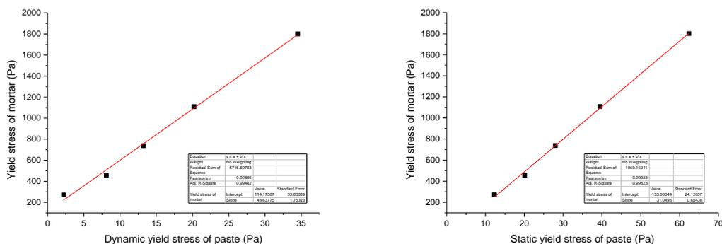
Figure 2: The fitting relationship between the yield stress of mortar and the dynamic and static yield stress of paste
