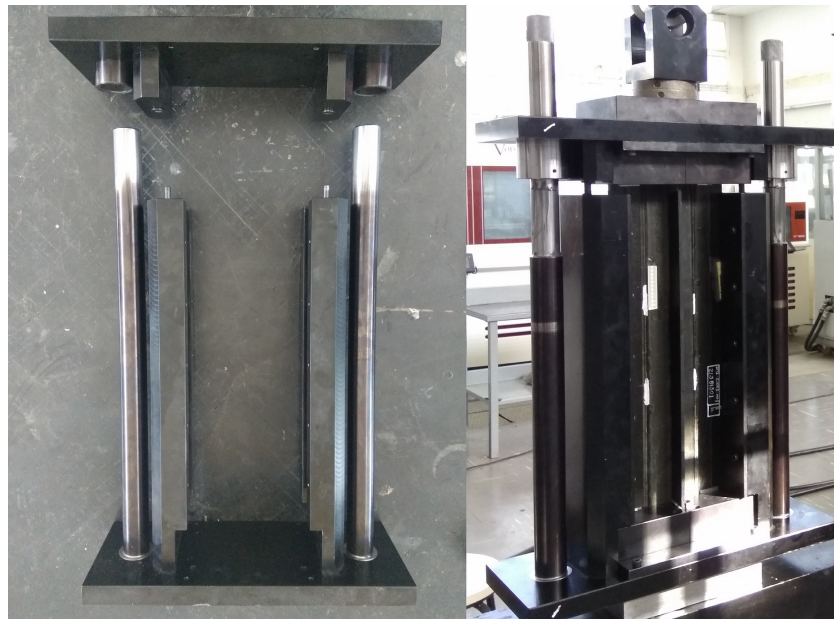
Figure 6.5: Left: initial test rig with signs of wear on the guiding rods. Right: modified test rig with knurled guide rod extensions and linear bearings installed.
