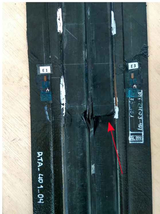
Figure 9.4: Skin failure, crippling of stiffener flange (marked by red arrow) and crushing of stiffener web. Panel ID:401_04
