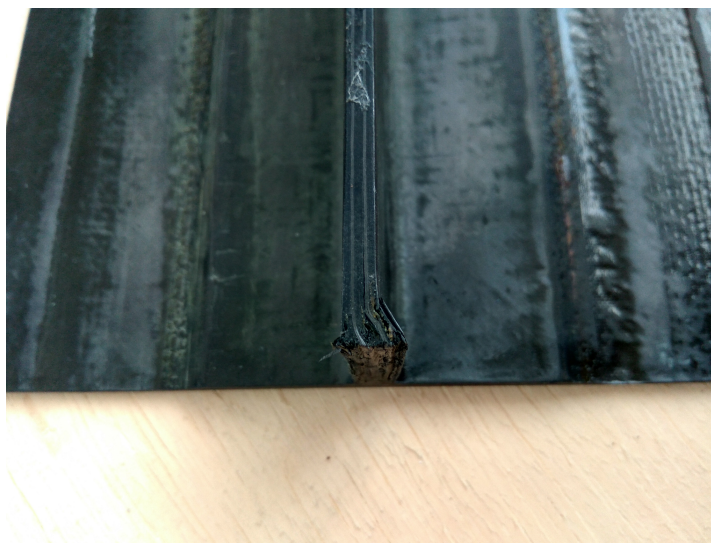
Figure 9.2: Crushing of stiffener clamped end. Panel ID:401_05
