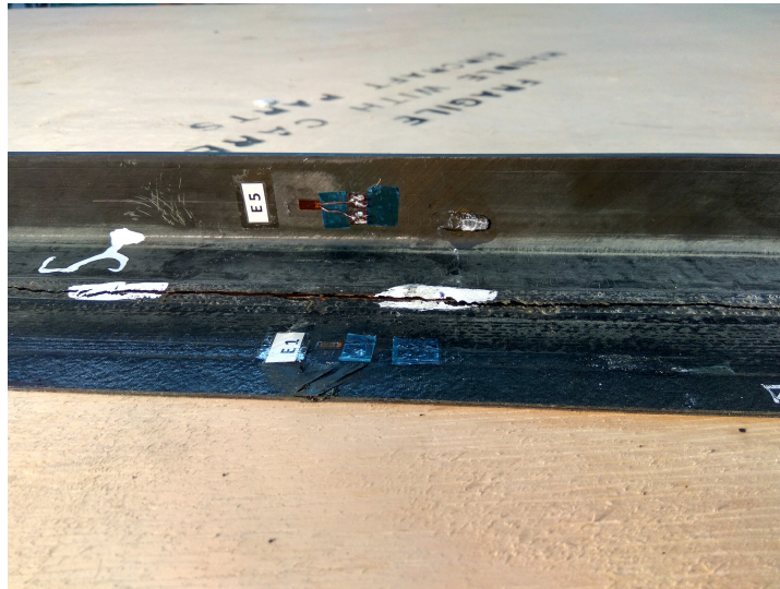
Figure 9.3: Delamination growth and skin failure. Panel ID:401_05
