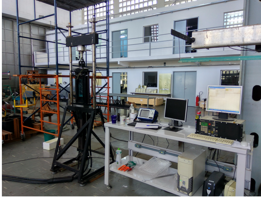
Figure 6.3: Fatigue test setup. Left to right: Load frame with test rig, portable c-scan device, hydraulic control computer.
