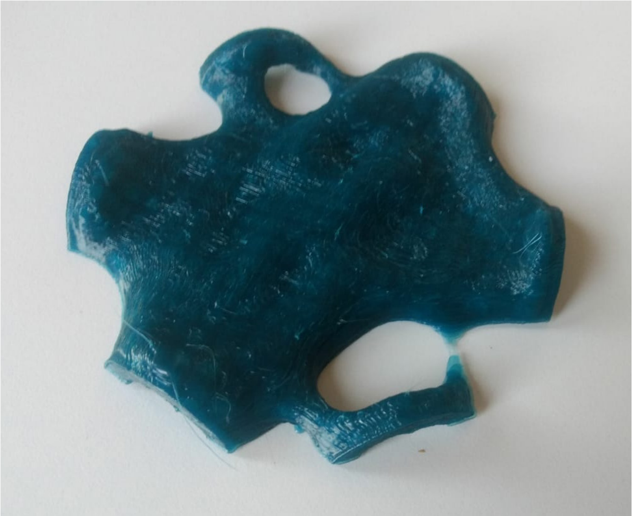
Fig. A14 Printing in layers, to reduce shrinkage and minimise the amount of support material required
