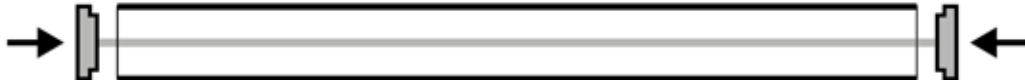
Fig. 65 Schematic of the new beam assembly, using minimised POM elements as interlayer and assembly component
