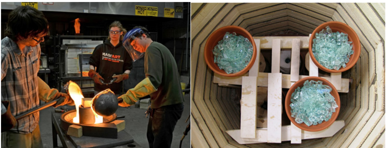
Fig. 8 Two methods of glass casting. Left, hot pouring, or melt-quenching. Pre-molten glass is taken out of a furnace (seen in the background) and poured into a mould. Right, kiln casting. Shown is the oven with the glass in ceramic pots and the moulds placed beneath. Heating the oven will cause the glass to melt and pour into the moulds.
