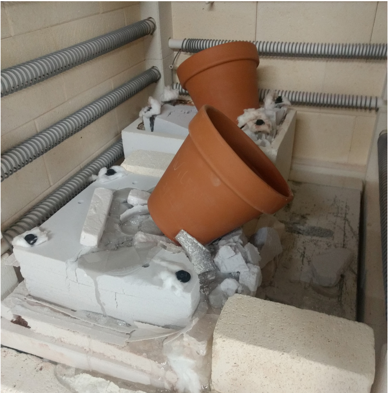
Fig. 143 The sand mould casting after the oven had cooled. In the foreground, the mould of the optimised node.
