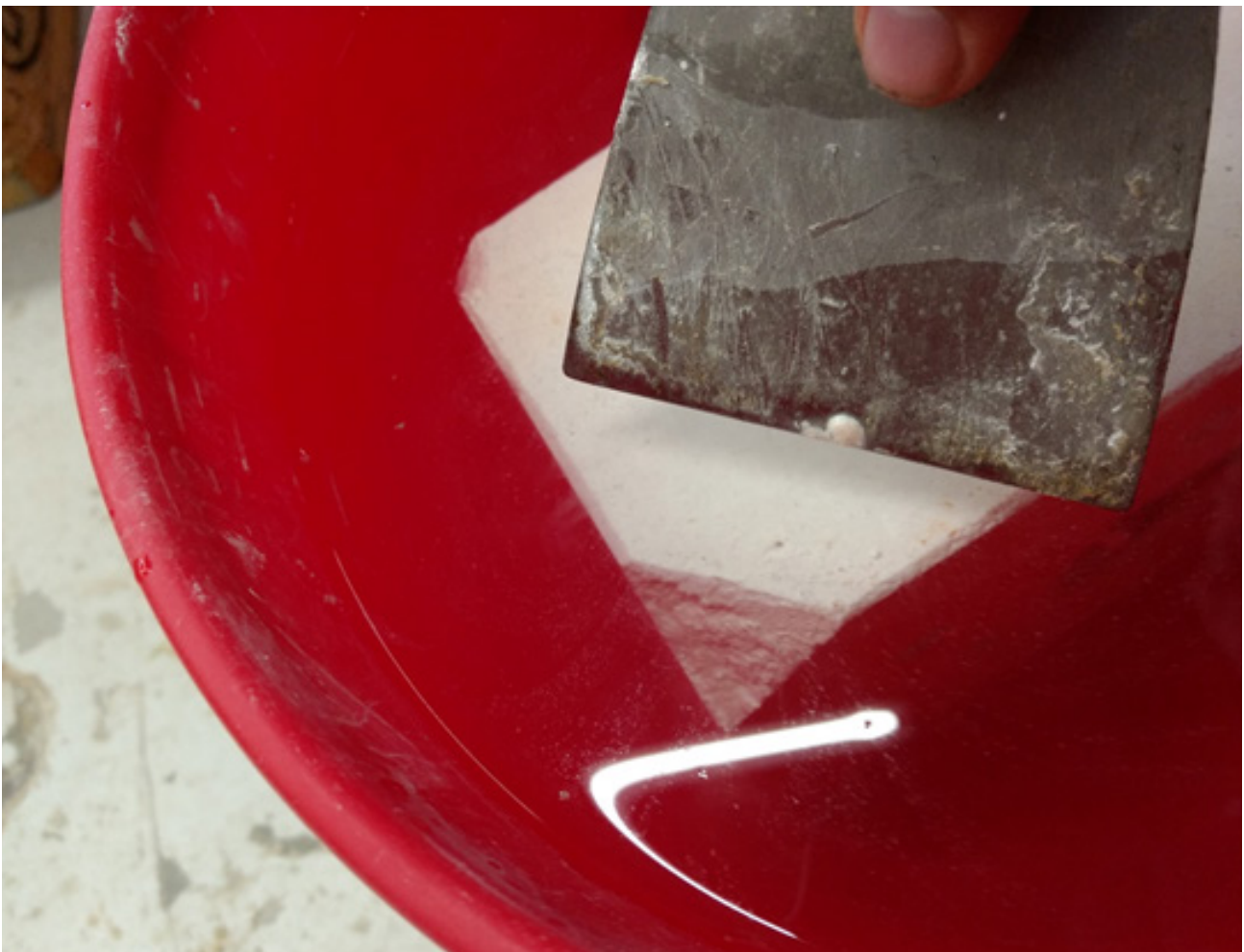
Fig. 138 Demoulding the lost wax cast. The silica mould becomes soft after submerging it in water
