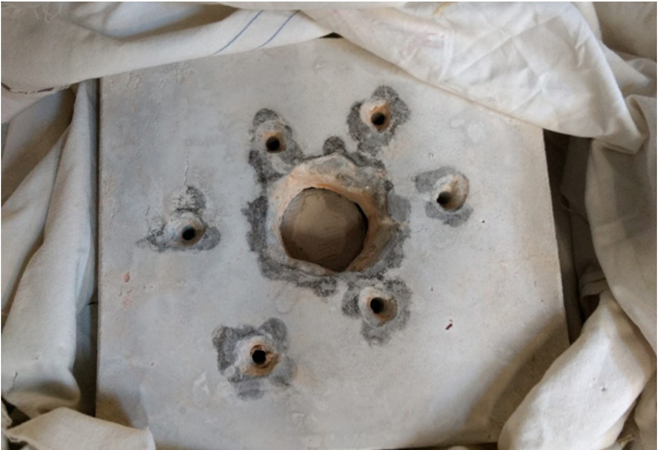
Fig. 136 The clean silica-plaster mould after the wax was burned out
