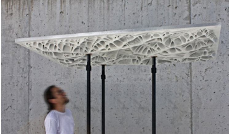
Fig. 27 ETH Zurich TO designed concrete slabs. Left, the slab that was calculated using the free Millipede software to be supported on three points. On the right, the slab calculated using professional ABAQUS software, to be supported at the four corners.
