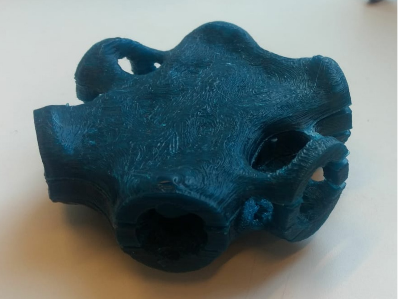
Fig. A15 Assembled layers. Some warping has occurred, causing large seams between the layers
