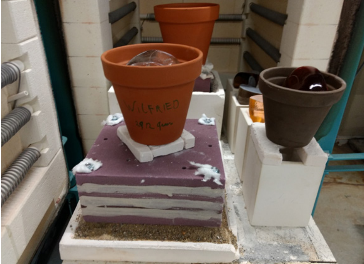
Fig. 131 Setup for the kiln casting. The flower pot with the needed amount of glass is placed on the sand mould
