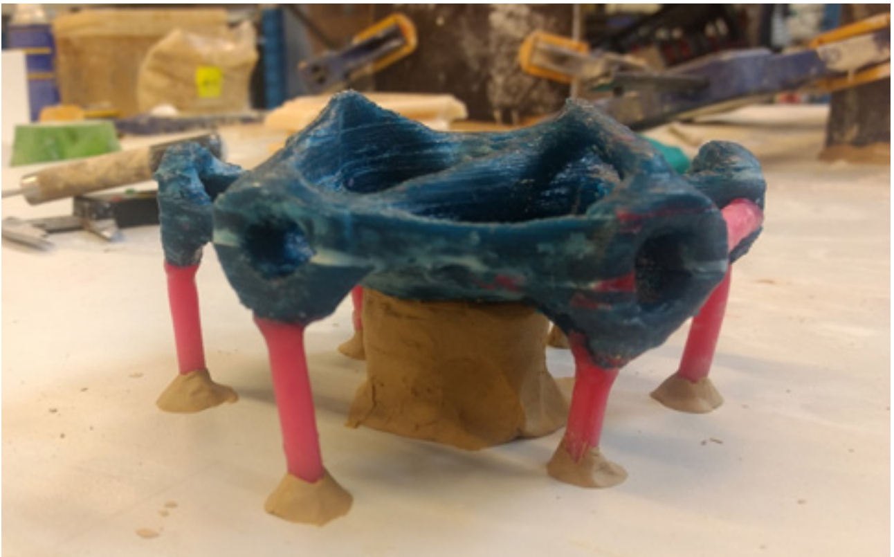
Fig. 133 Mould setup, with added elements for casting in wax and clay
