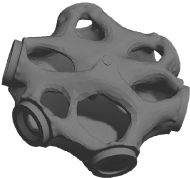
Fig. 93 Geometry after shrink-wrapping and smoothing
