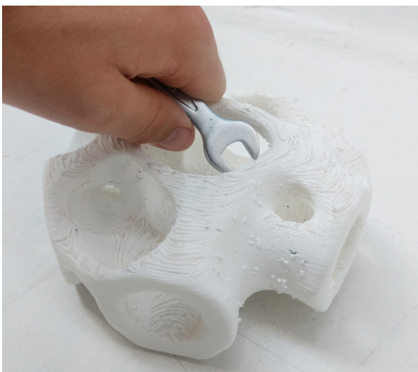
Fig. 96 Small scale of optimised element makes assembly complicated
