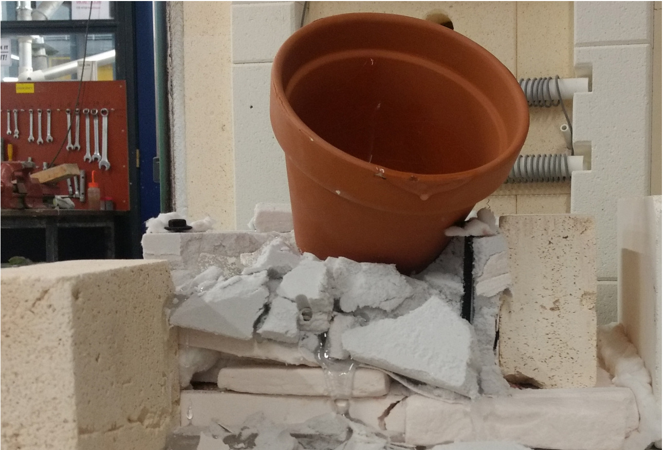
Fig. 144 Collapse of the mould, seemingly caused by the weight of the glass-filled flowerpot
