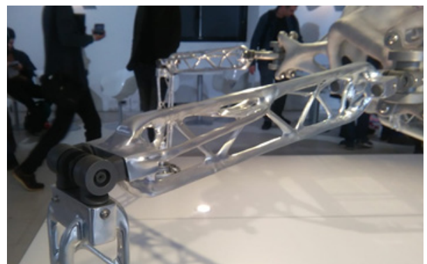
Fig. 57 Leg of the Autodesk/JPL optimised lander. A similar optimised geometry fabricated in glass can be imagined for the beams of the shell pavilion
