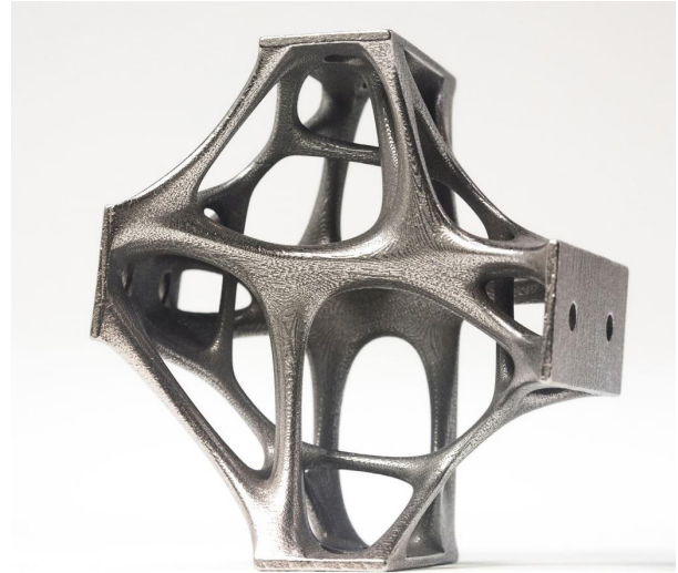
Fig. 39 Finalised node produced using direct laser metal sintering. Prayudhi, 2016
