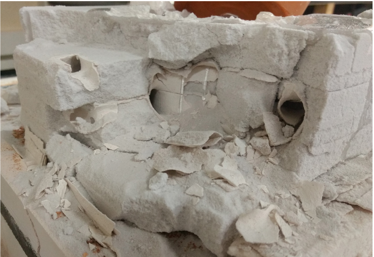
Fig. 145 The thin interior layers formed by the silica-plaster coating, have stayed intact where the mould was not crushed by the flowerpot.
