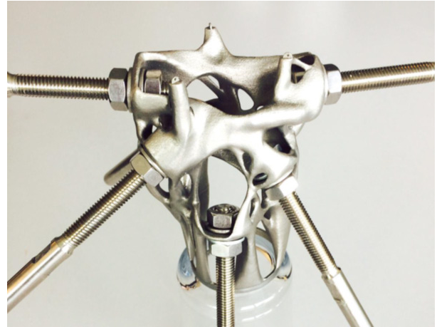
Fig. 55 Close-up of the ARUP node with integrated connections
