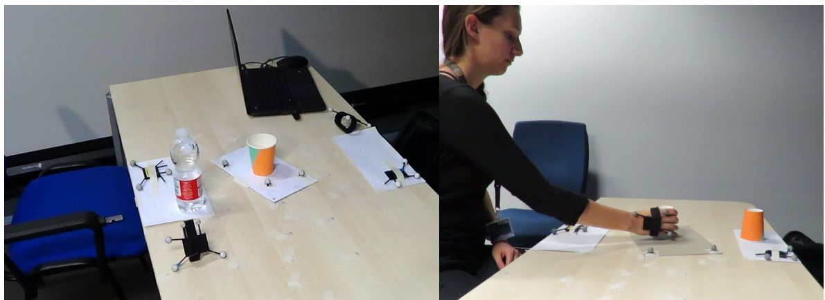
Figure 5.1: Setup used to record the demonstrations. Three local frames were attached to the table, the local frame for the human perspective, the local frame for the robot and one for the perspective of the object. One OptiTrack marker was attached to the back of the hand to record the movements.
