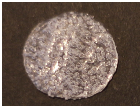
Figure 4.10: Bubbles formed in PVB reference membrane.
