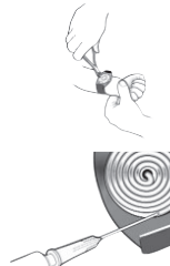
USE TWISTING MOTION WHILE INSERTING BLUNT NEEDLE INTO THE END OF THE MICRO-BORE TUBING.
