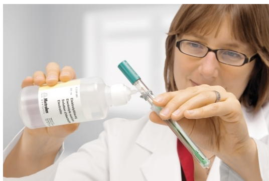
Figure 4.9: Commercially available reference electrode for use on all electrochemical cells filled with a electrolyte solution [61].
