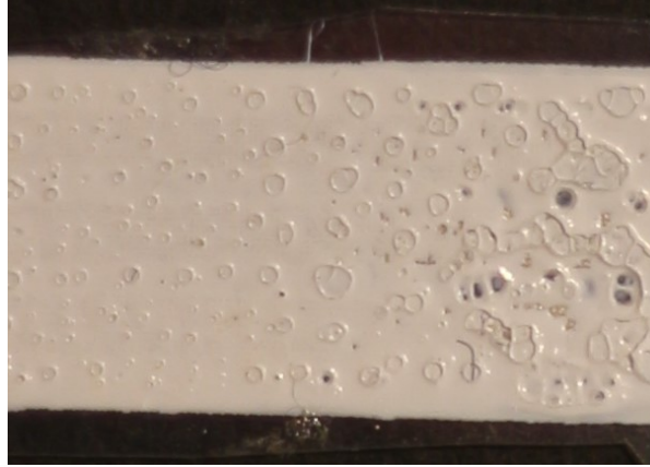
Figure 4.8: Bubble formation in dielectric ink.
