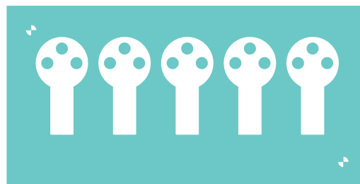
Figure 4.7: Screen-printing layer 4 of sensor design V3.
