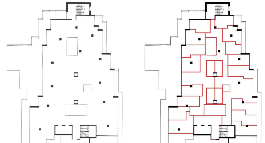
Fig. 3: Floorplan of La Mémé. With and without adaptable parts. (underlay from: Kroll, 1990, p. 37)
