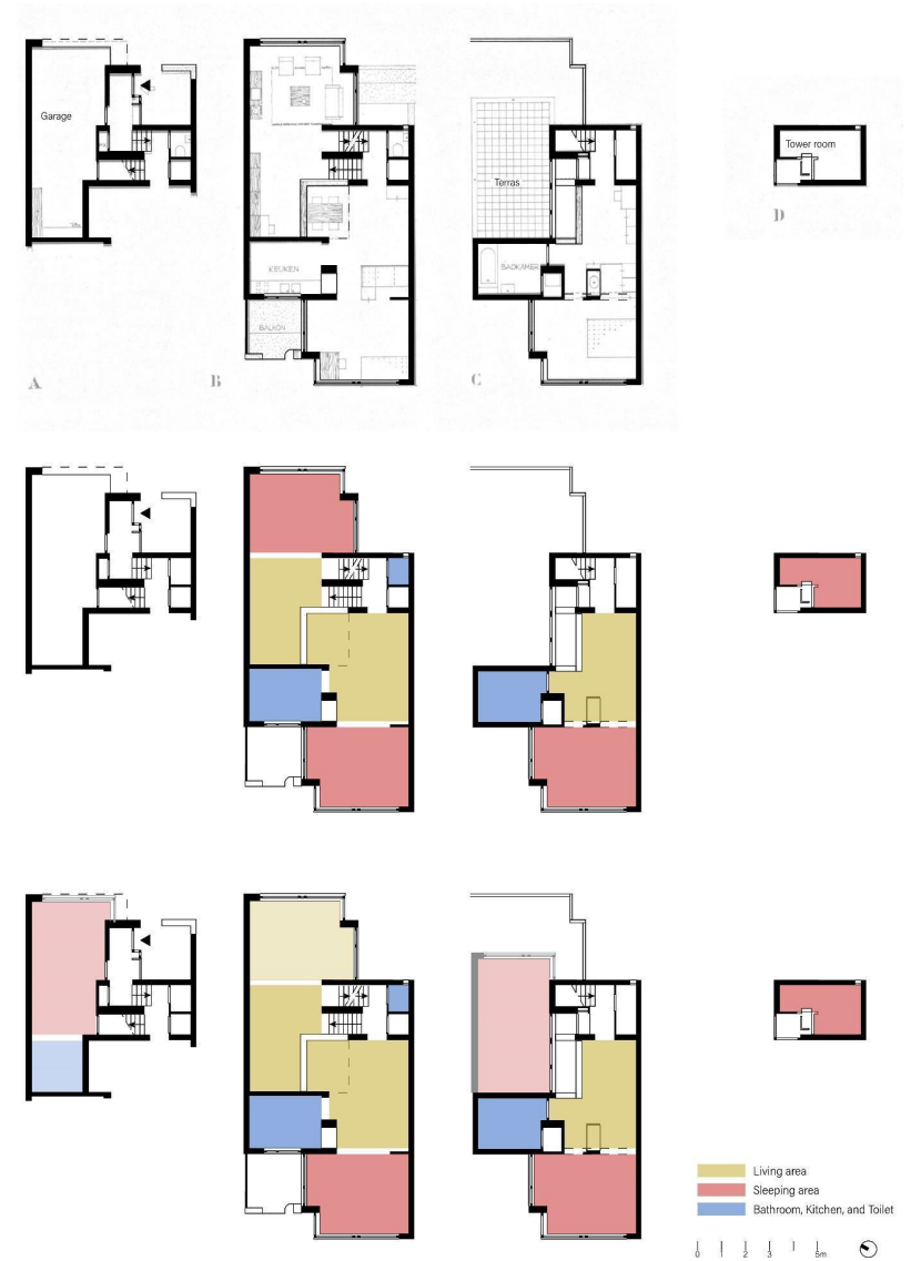
Fig. 8: Designed floorplans (top), functions in the 1970s (middle), and present expansions and functions (bottom). (drawings based on floorplans from https://www.architectuur.nl/project/diagoonwoning/ )
