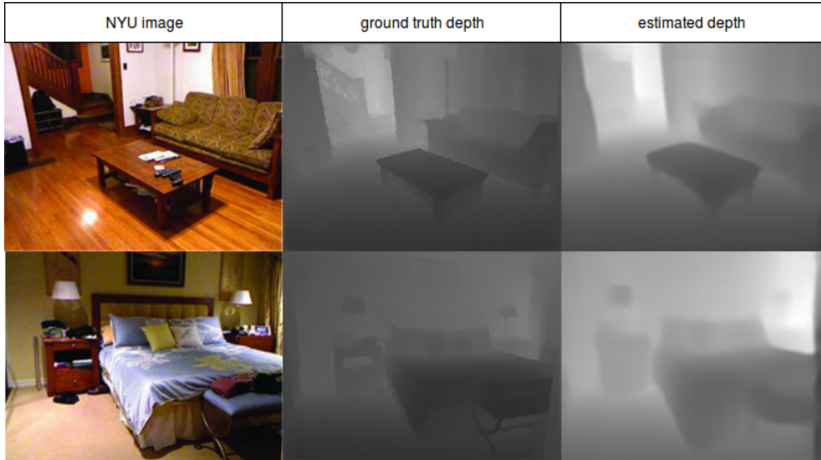
Figure 3.4: Examples of images from the NYU dataset, together with the ground-truth depth-map and the depth-map estimated by the CNN trained on the NYU dataset.
