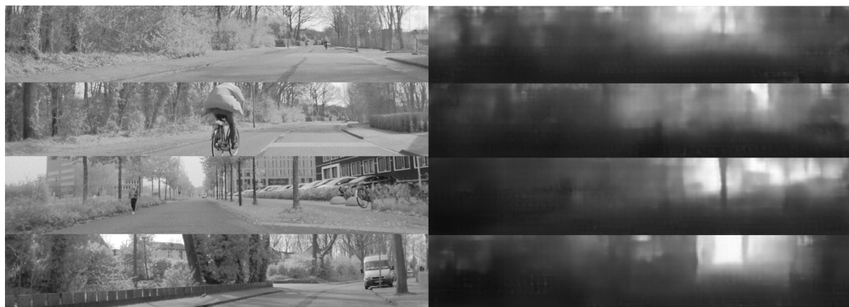
Figure 4.13: Left: The WEpod images cropped to the same aspect ratio as the Kitti images with the horizon in the middle. Right: The resulting estimated depth image.
