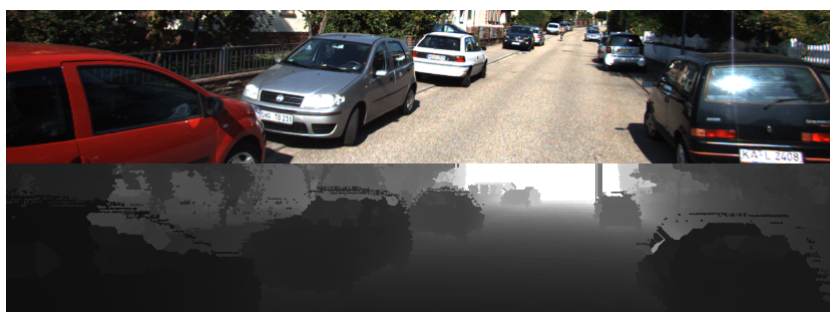
Figure 3.6: An example image and its dense depth-map created by the linearly interpolating projected 3D lidar points from a 64-plane lidar. The image has been cropped to a height of 228 to only contain the area that the lidar points cover.
