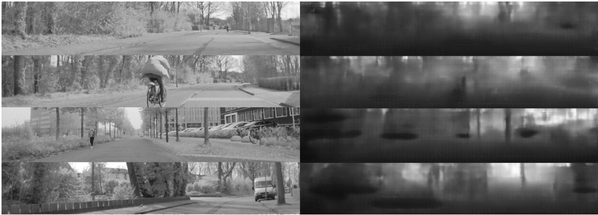
Figure 4.14: Left: The WEpod images cropped to the same aspect ratio as the Kitti images with the horizon in the middle and resized to the same size. Right: The resulting estimated depth image.
