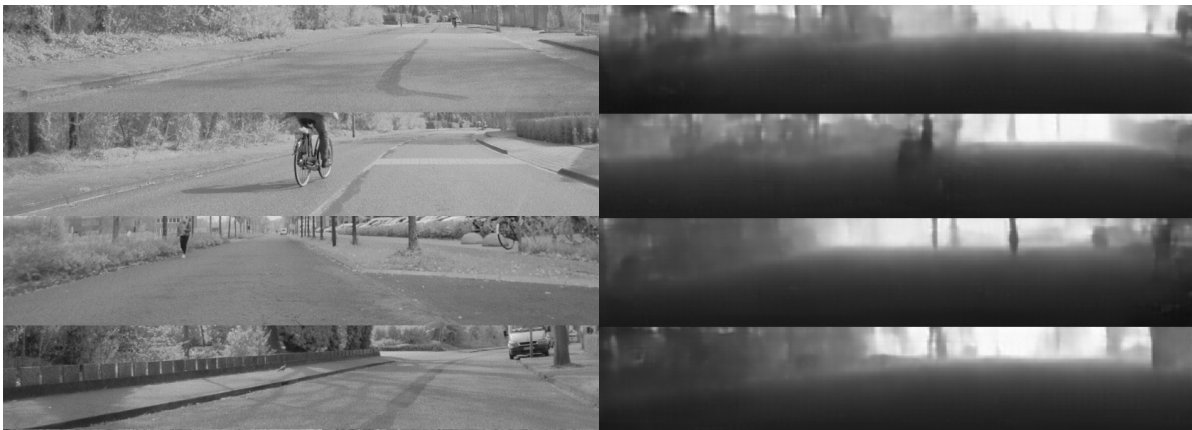
Figure 4.15: Left: The Wepod images cropped to the same aspect ratio, with the horizon at the same height and resized to the same size as the Kitti images. Right: The resulting estimated depth image.
