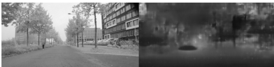
Figure 4.12: Left: The input WEpod image. Right: The resulting output depth image form the CNN trained with L2 loss, trained for 25 epochs with lr0.0001epd1dr0.95.
