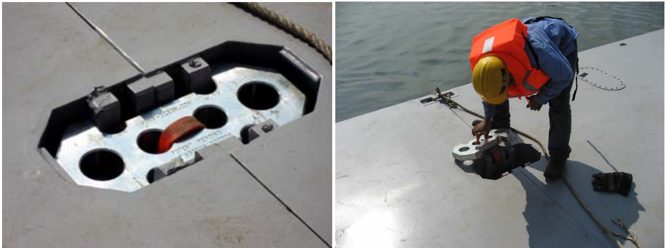
Figure 3: Hann-Ocean rigid pontoon connector
